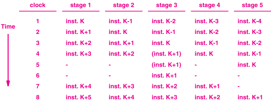
Figure 5.5 Illustration of a pipeline stall. Instruction K+1 cannot proceed until operand C becomes available.
