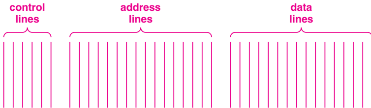
Figure 14.4 Conceptual division of wires that comprise a bus into lines for control, addresses, and data.
