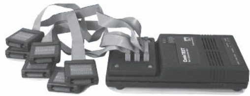
Figure 15.8: CodeTest software performance analyzer for real-time systems. Courtesy of Metrowerks, Inc.
