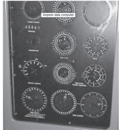
Figure 1.8: An analog computer from a WWII submarine. Photo courtesy of www.fleetsubmarine.com .
