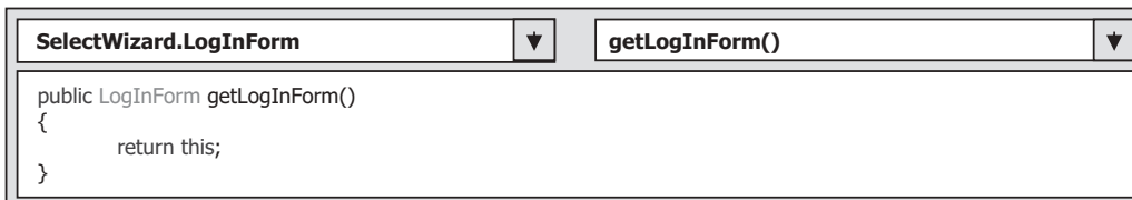
Figure 5.45 Coding for the getLogInForm method.
