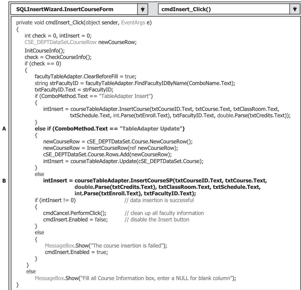
Figure 6.41 Code modifications for the Insert button's Click method.
