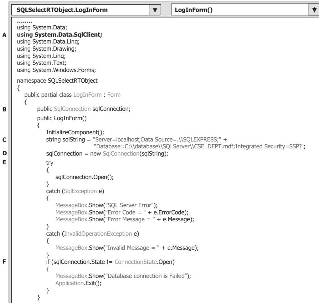
Figure 5.107 Coding for the database connection.
