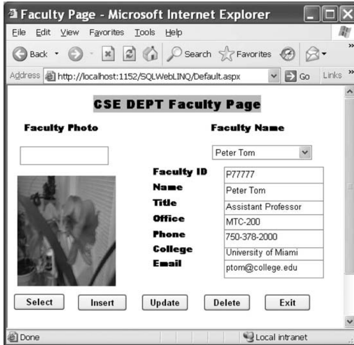
Figure 8.56 Testing status of the data insertion action.
