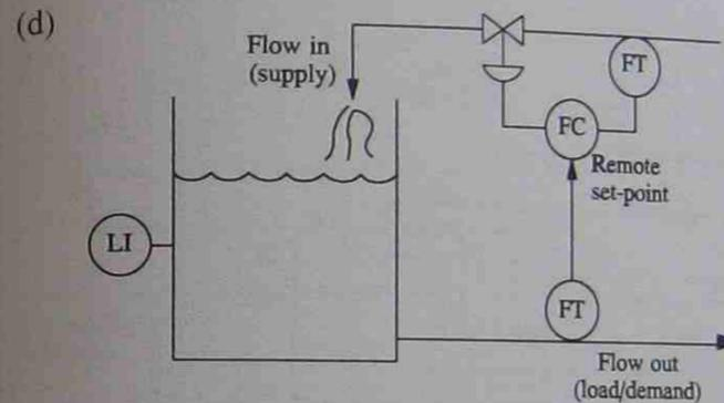
*Note:* The system shown above, achieves a stable level by measuring demand, and matching supply (flow in) with demand (flow out). i.e. when flow in = flow out, the level must be stable.
