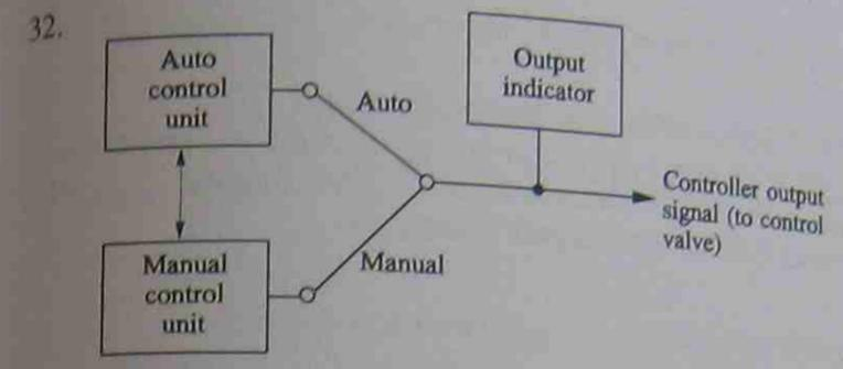
When switching between auto and manual, the controller output should *not* change, otherwise there will be a change in control valve position and a disturbance to the process, (A 'bump'). The 'bumpless transfer' function operates to make the auto output follow the manual output when on manual, and makes the manual output follow the auto output when on auto. Thus when switching between auto and manual, the controller output will not change.
