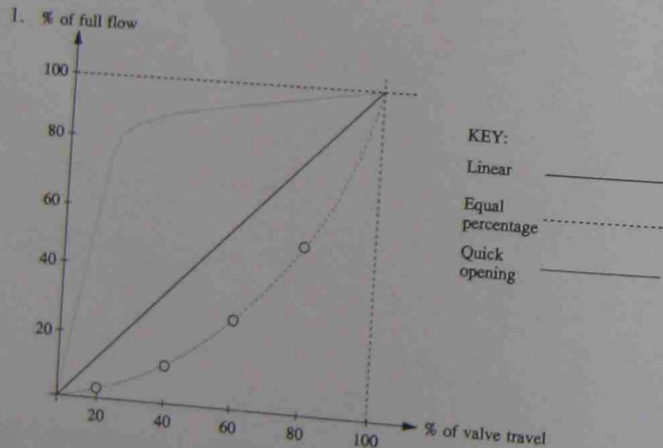
2. Inherent characteristic - This is determined under condition of a constant pressure drop across the valve for all values of flow and valve travel from 0 to 100%.
