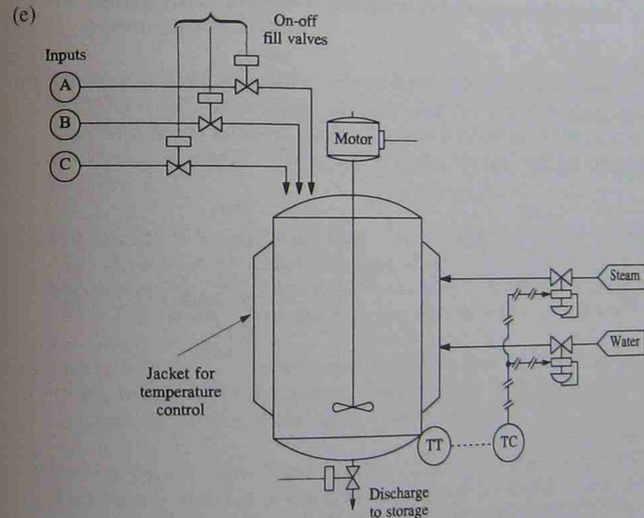
(f) The feedback temperature control loop provides continuous temperature control during the processing phase of the batch cycle.
