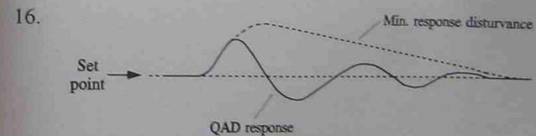
17. QAD - The QAD (or minimum area) response is commonly used on most control loops. The QAD response returns the PV back to the set point in the minimum possible time, with the least waste of energy. However the QAD (Quarter Amplitude Damped) response cycles for three to four cycles before the PV stabilises again.
