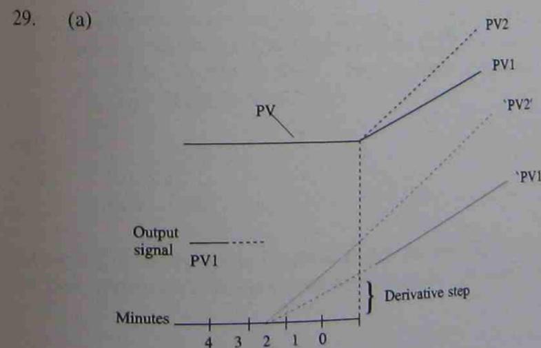
(b) As shown in the diagram proportional action appear to have occurred two minutes prior to the change in the recorded process variable. Due to control loop lags, the recorded change will lag the actual process (PV) change. Thus derivative action as shown, attempts to compensate for time lags in the control loop.
