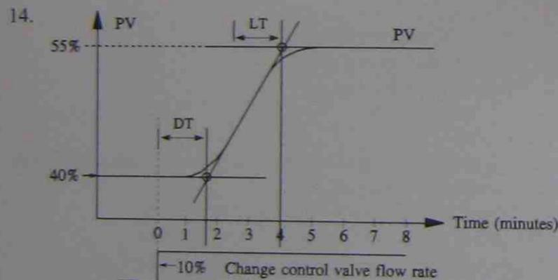
$$DT = 1.6 \text{ mins} \quad LT = 2.4 \text{ mins (obtained from graph).}$$
