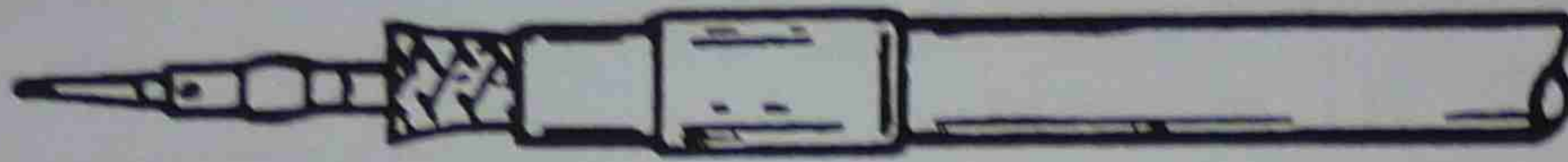
Figure 75 Assembling centre pin
