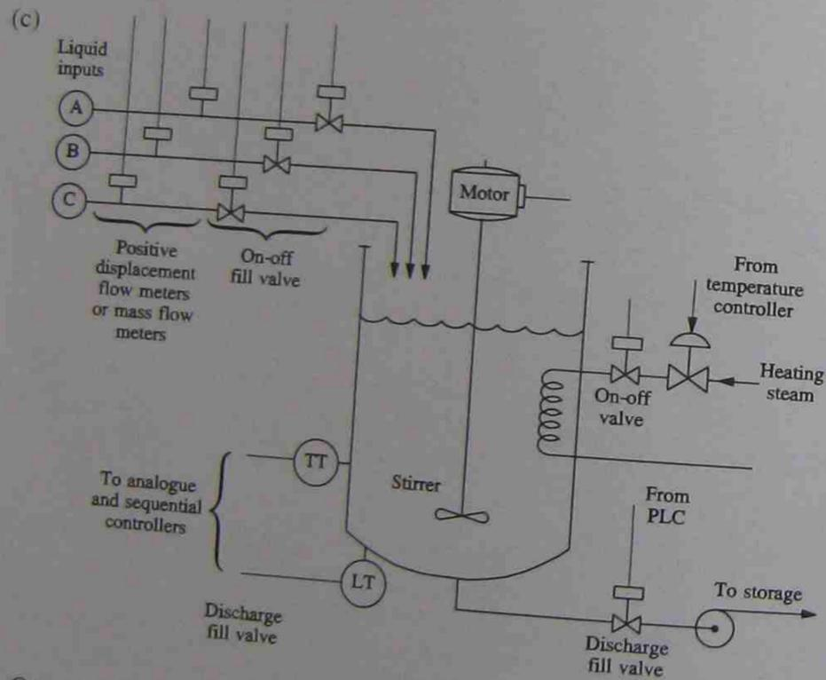
Operation - The required quantities of liquids A, B and C are measured by the flowmeters and the PLC then shuts the on-off fill valves, in the required sequence (and stops the fill pumps, not shown).
