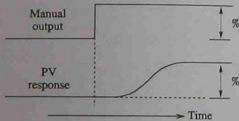
(b) Remove the response curve obtained from the chart recorder.
