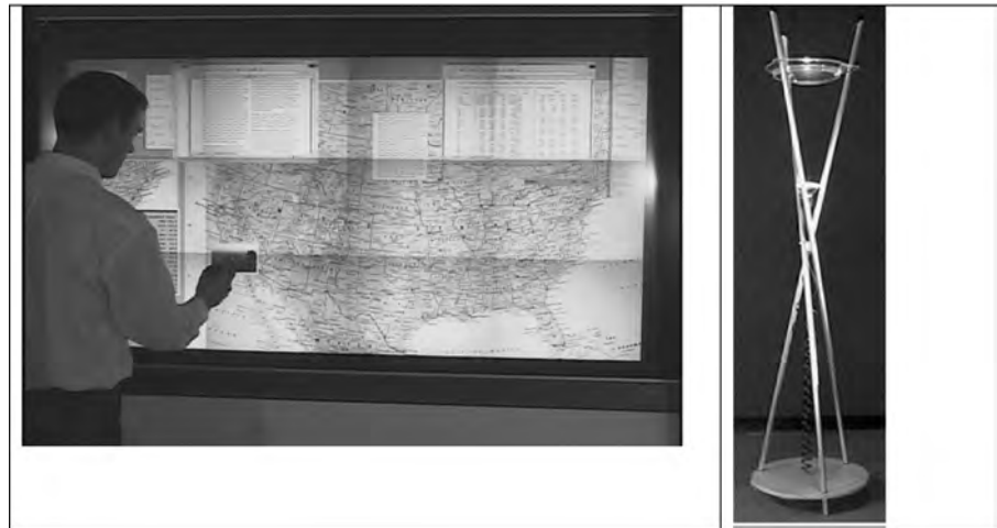
Figure 20.3 The figure on the left is the Stanford Interactive Mural, an example of a large-scale interactive display surface created by tiling multiple lower-resolution projectors. Picture courtesy François Guimbretière. The figure on the right is an example of an ambient display, the Water Lamp from Ishii's Tangible Media Group at the MIT Media Lab. Light shines upwards through a pan of water, which is actuated by digitally controlled solenoids that can tap the water and cause ripples. External information can be used to drive the tapping of the solenoids. Source: Courtesy of Hiroshi Ishii, MIT Media Lab. Photograph by Andrew Daly
