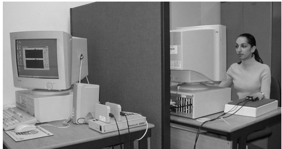
Figure 9.7 Data Lab Psychophysiology equipment showing some of the sensors (above) and a typical experimental arrangement (below) with sensors attached to the participant's fingers and the monitoring software displayed on the evaluator's machine. Source: Courtesy of Dr R. D. Ward
