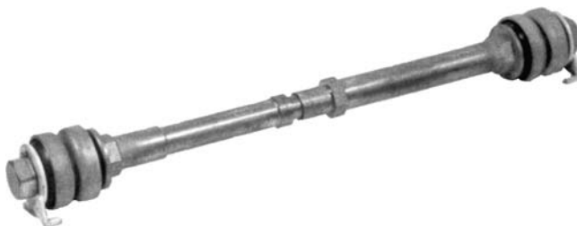
FIGURE 3.21 Trailing arm suspension on a Y32 bogie.
