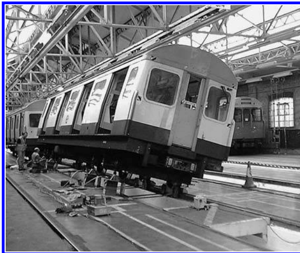
FIGURE 13.32 Sway test. Source: Photo — courtesy of Serco Railtest Ltd.
