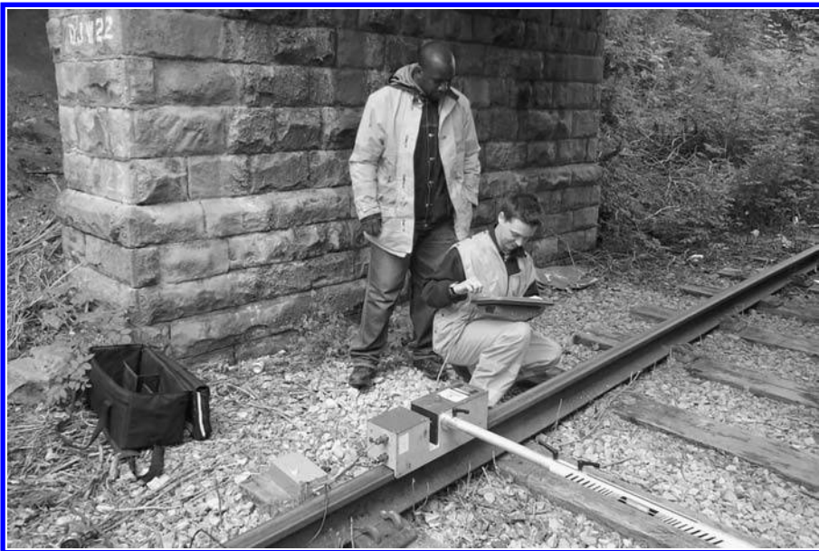
FIGURE 7.4 The LaserSweep profiler.
