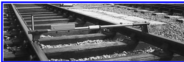
FIGURE 13.24 Cant and gauge stick (courtesy of Abtus Ltd.). Source: Abtus Ltd. — Catalogue. With permission.
