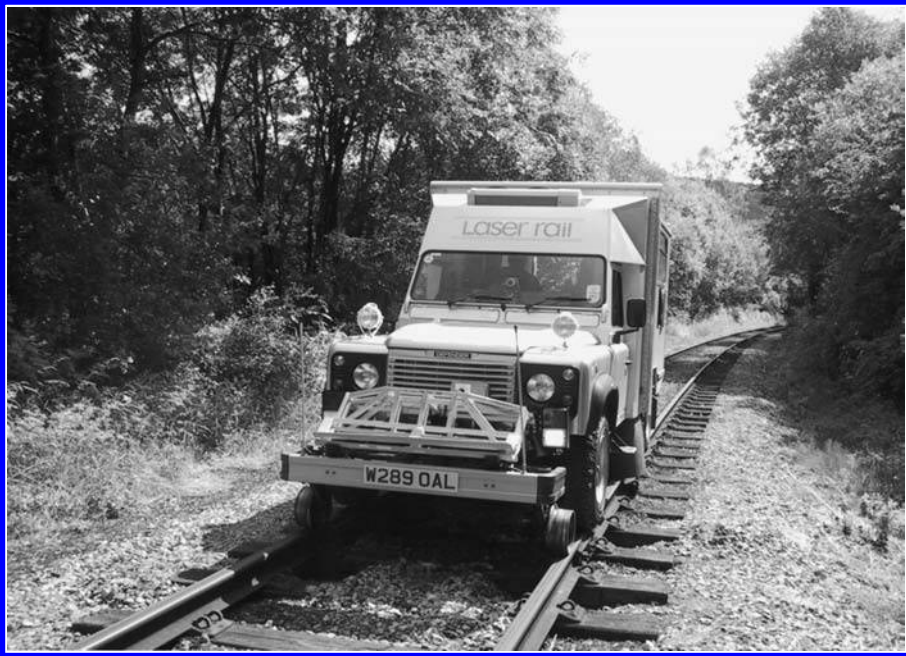
FIGURE 7.5 Road–Rail laser gauging vehicle, operated by Laser Rail Ltd.
