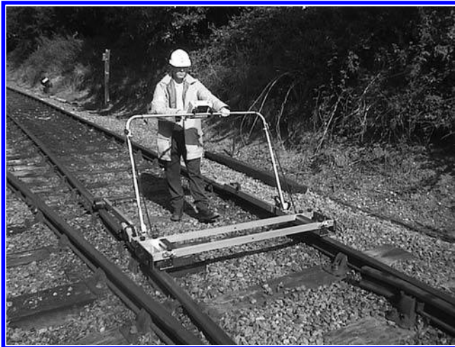
FIGURE 13.25 Track geometry recording trolley (courtesy of Abtus Ltd.). Source: Abtus Ltd. — Catalogue. With permission.
