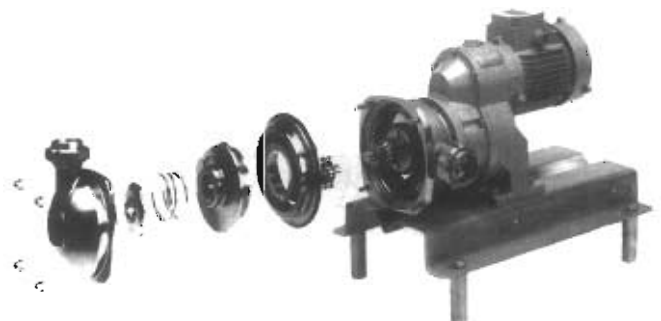
Figure 1.88 Exploded view of an eccentric drive pump
