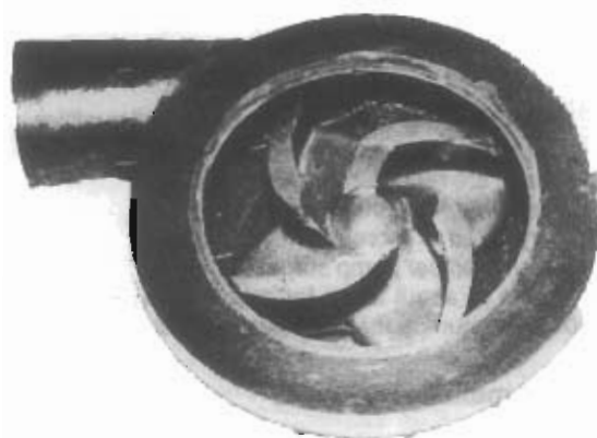
Figure 7.18 Pump impeller made of urethane coated steel and pump casing of solid urethane rubber
