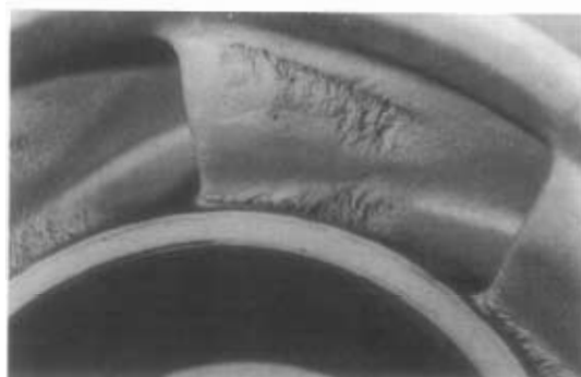
Figure 7.19 Typical cavitation damage of pump impeller
