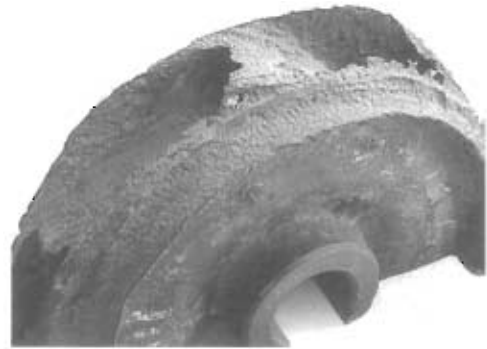
Figure 4.53 Severe cavitation damage to a centrifugal pump impeller
