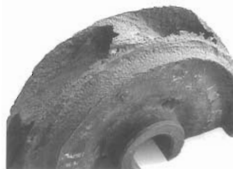
Figure 7.20 Severely damaged pump impeller
