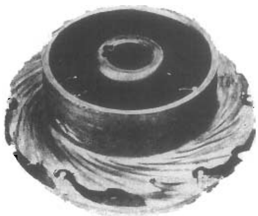
Figure 7.12 Erosion-corrosion on a 13Cr + Mo steel impeller
