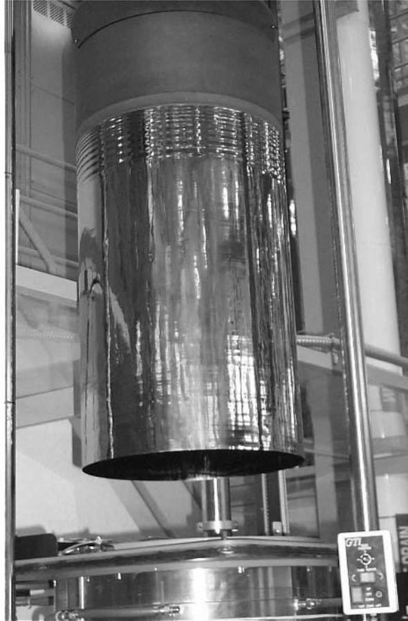
**Figure 6.23** Experimental 50-cm-diameter EFG cylinder exiting from furnace
