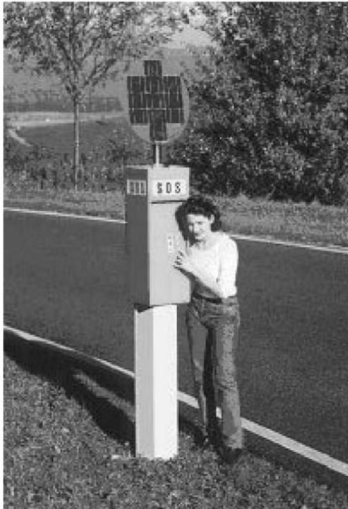
**Figure 2.13** Autonomous emergency phone and information system using photovoltaic power supply
