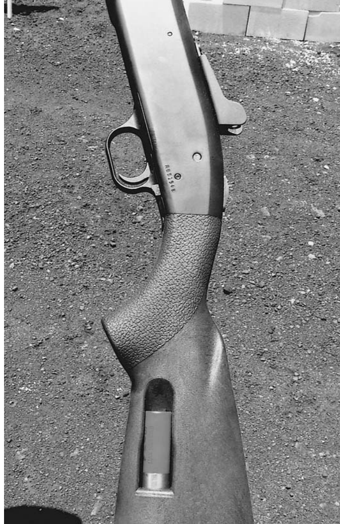
The pistol grip area of the 590 has a mottled finish that is meant to offer a more firm hold when firing. The Speedfeed feature holds two additional three-inch Magnum shells on each side of the stock for fast reloading.
