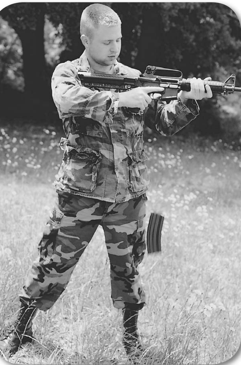
For rapid reloading with a fresh magazine, one simply has to push the magazine release button and the empty falls out, saving seconds in the process.
