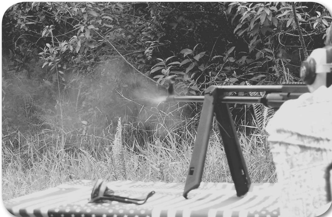
The hand guard of the carbine is of a heavy-duty man-made material. It can be unsnapped and swung down to form a bipod. Note the gases from the muzzle when fired.
