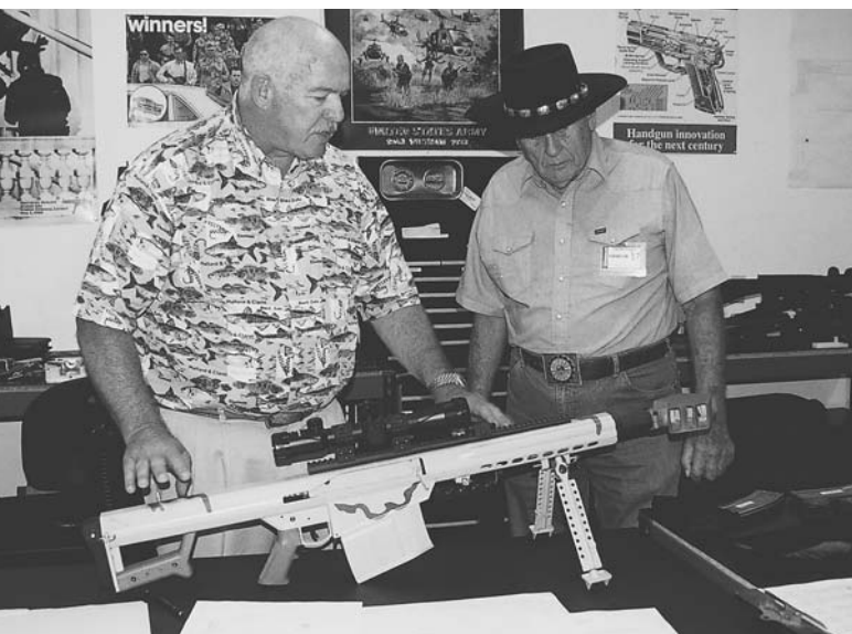
Bob Gates, Barrett vice-president, explains the workings of the XM109, a new rifle that is designed to fire a 25mm cartridge against materiel targets.
