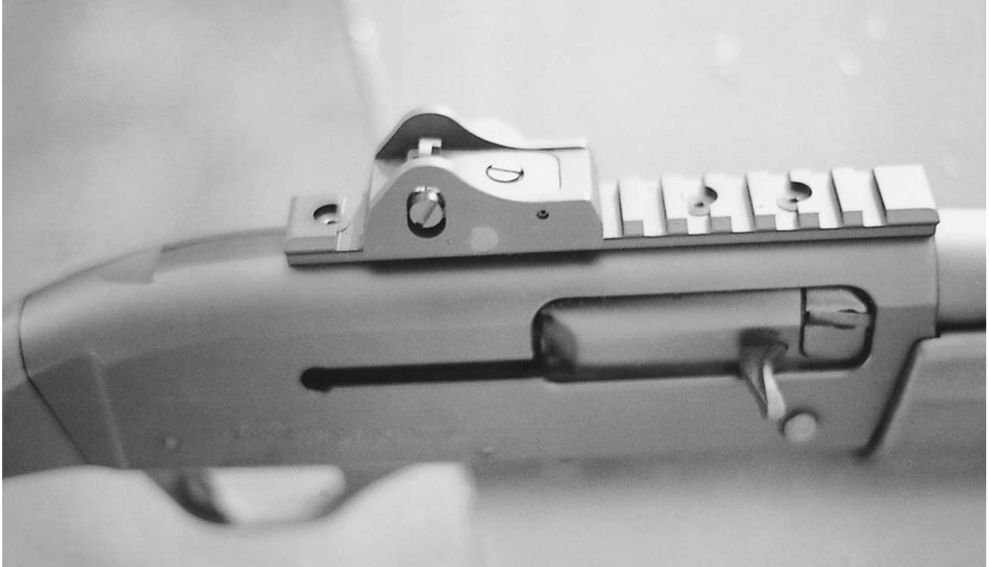
The rear sight of the FN auto-loading shotgun is of the Ghost Ring-type that allows one to get on target in a hurry.
