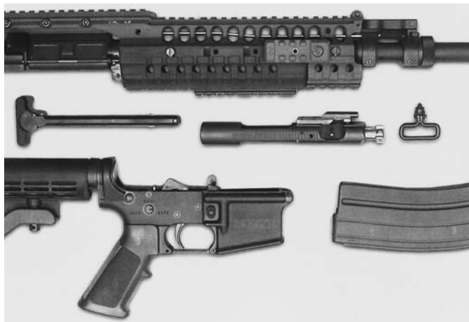
Field-stripping of the Barrett rifle for cleaning or repair is accomplished with ease. The M468 upper receiver can be replaced with one designed to fire the 25mm cartridge.
