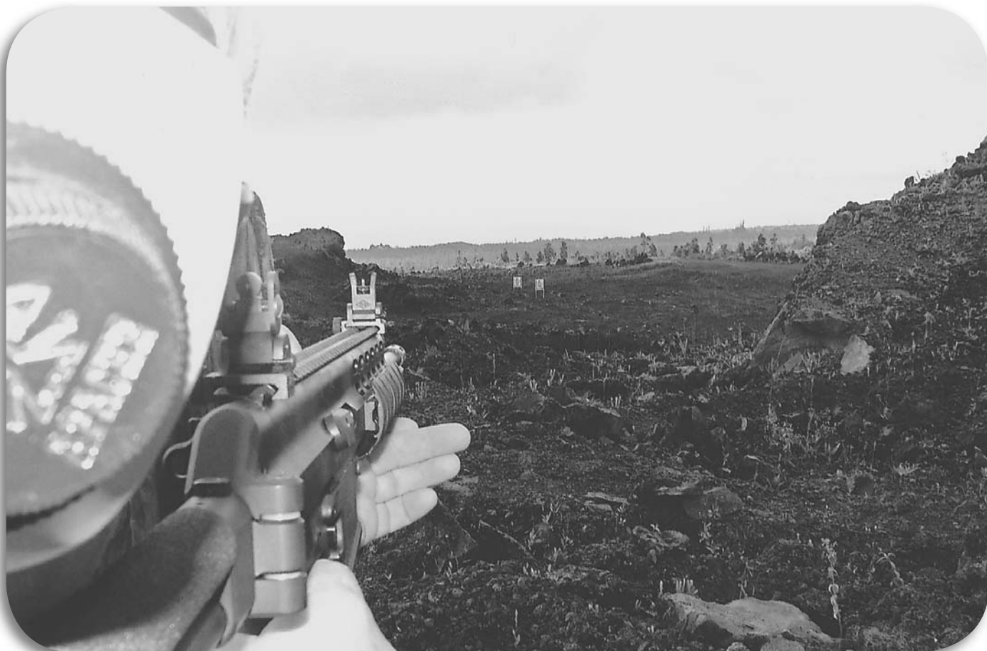
The sights of the rifle were attached to the machined rail, with the rear being adjustable for changes in elevation and windage.
