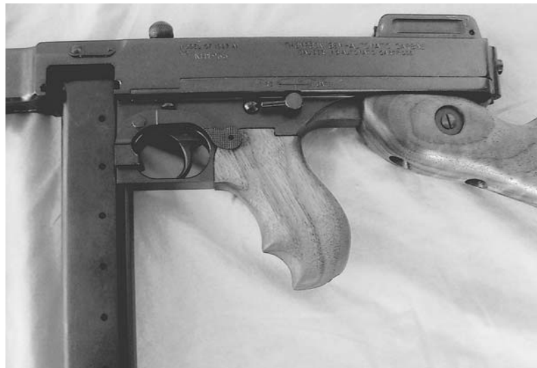
The bolt of the Thompson was actuated by the knob on top of the receiver. The 30-round magazine snaps into position easily.
