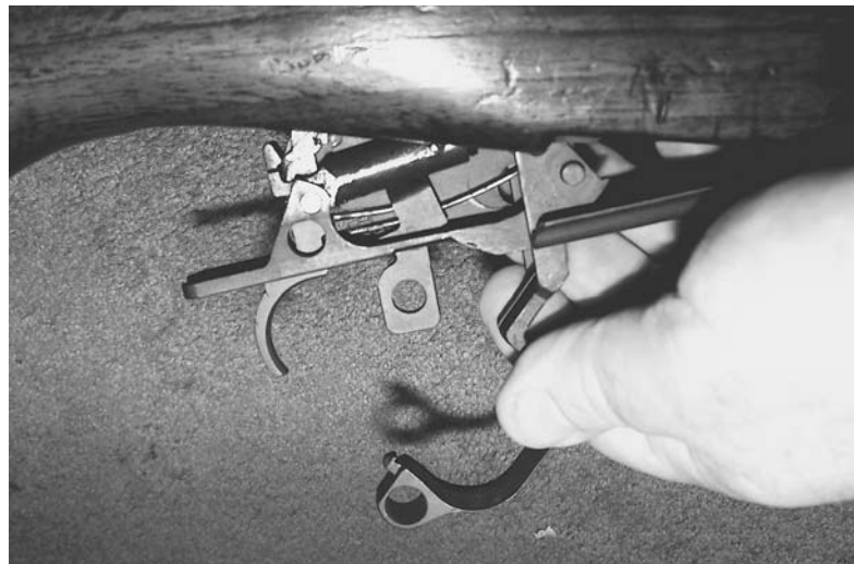
As designed by John Garand, the trigger guard swung open so the stock could be removed. Note the safety with the hole in it for inserting a padlock during storage.
