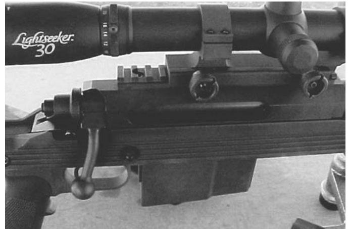
The test rifle was equipped with a rail that allowed quick attachment of a scope equipped with the proper rings and mounts.
