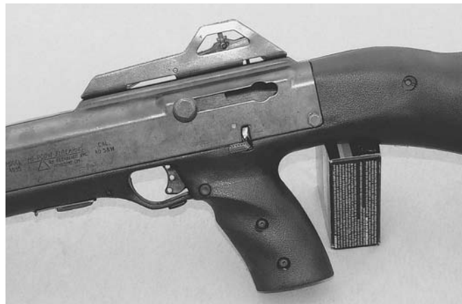
The controls for the U.S.-made carbine, including the cocking handle and the safety, are positioned on the left side of the firearm, all within easy reach for the shooter.
