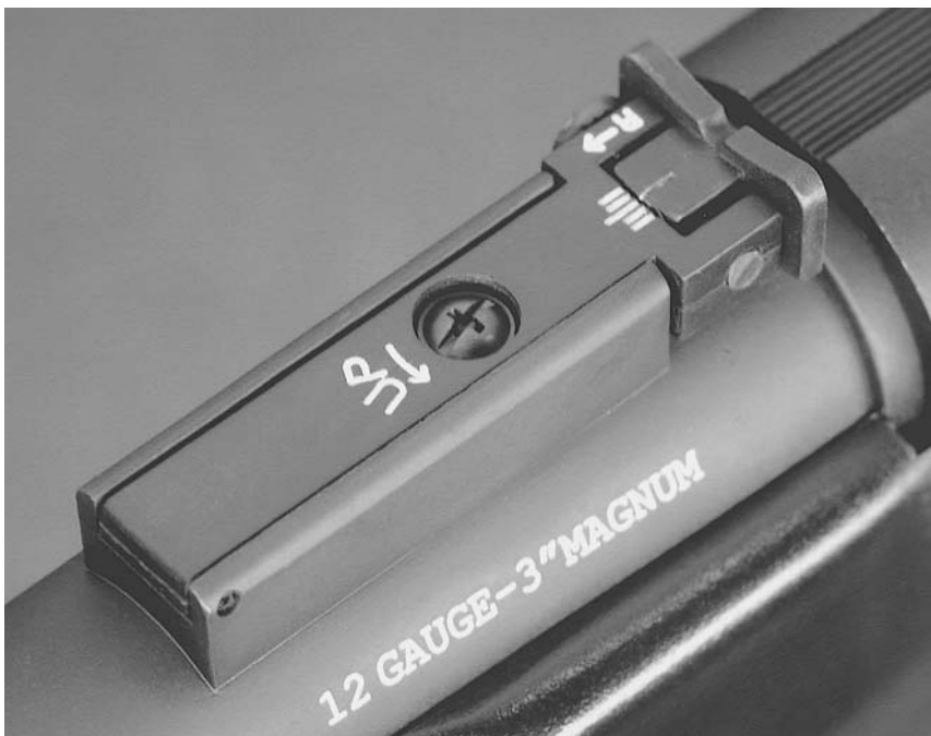
An 18-inch barrel is available for the Police Model Sabre with this precisely adjustable rear sight. Jack Lewis found it an aid to accuracy when firing slugs.
