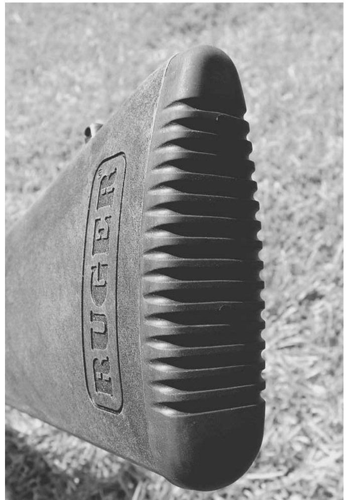
The butt of the Ruger carbine features a ridged pattern that is an aid in holding on target. The stock and forend of the firearm are cast from Dupont's Zytel.
