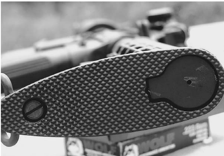
The stock of the carbine is hollow and is covered by a carbon composite butt plate. The trapdoor covers the compartment that can hold cleaning gear.
