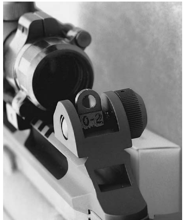
The rear sight of the carbine is moulded as a part of the carbon composite rail. The flip-type aperture was developed to handle two different ranges.
