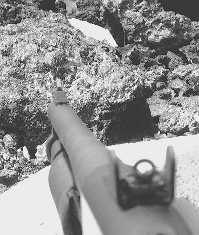
The Ghost Ring-type rear sight is fashioned from what appears to be a steel stamping, but it is well protected by heavy metal ears. The front sight carries a red insert for fast target-alignment.
