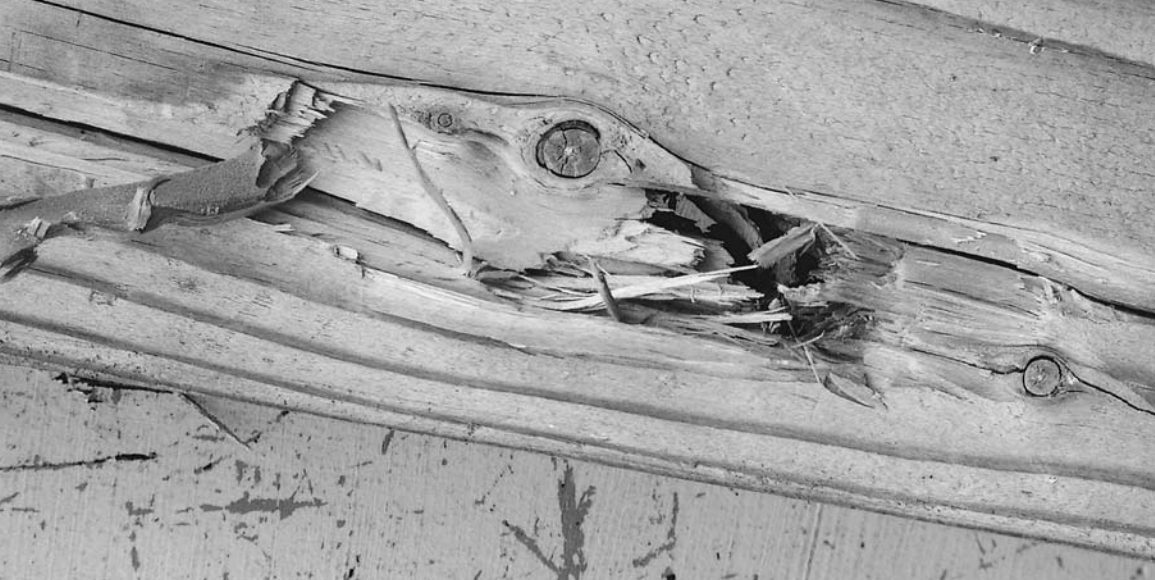
When the rear of the plywood test target was checked, it was found that the sabot-type slug damaged the wood badly after passing through.
