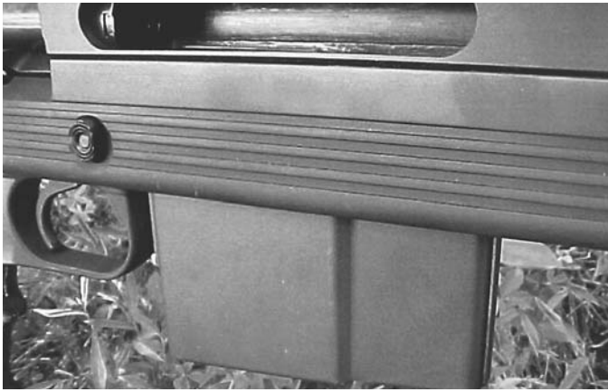
The magazine of the ArmaLite-built gun carries five rounds of 338 Lapua Magnum ammunition. Note the magazine release directly above the trigger, making it easier and faster to change magazines.
