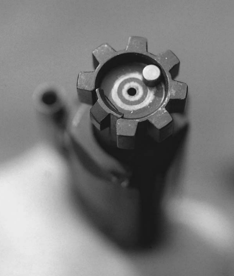
One also should be sure to clean the bolt face. Foreign matter may work its way into the firing pin channel and cause a weak strike.
