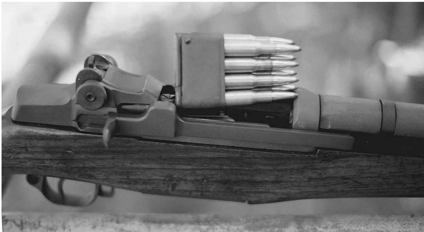
The Garand en block clip could be loaded from either side, a feature that was considered laudable for faster reloading of the rifle in combat.
