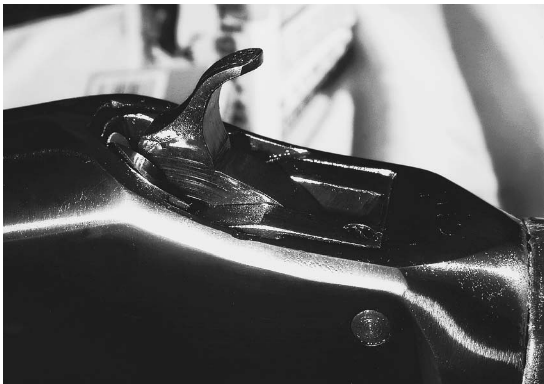
While overall machining of the Norinco clone was adequate, Lewis found tool marks on small parts like the hammer. He recalls his family's original as being perfect, of course.
