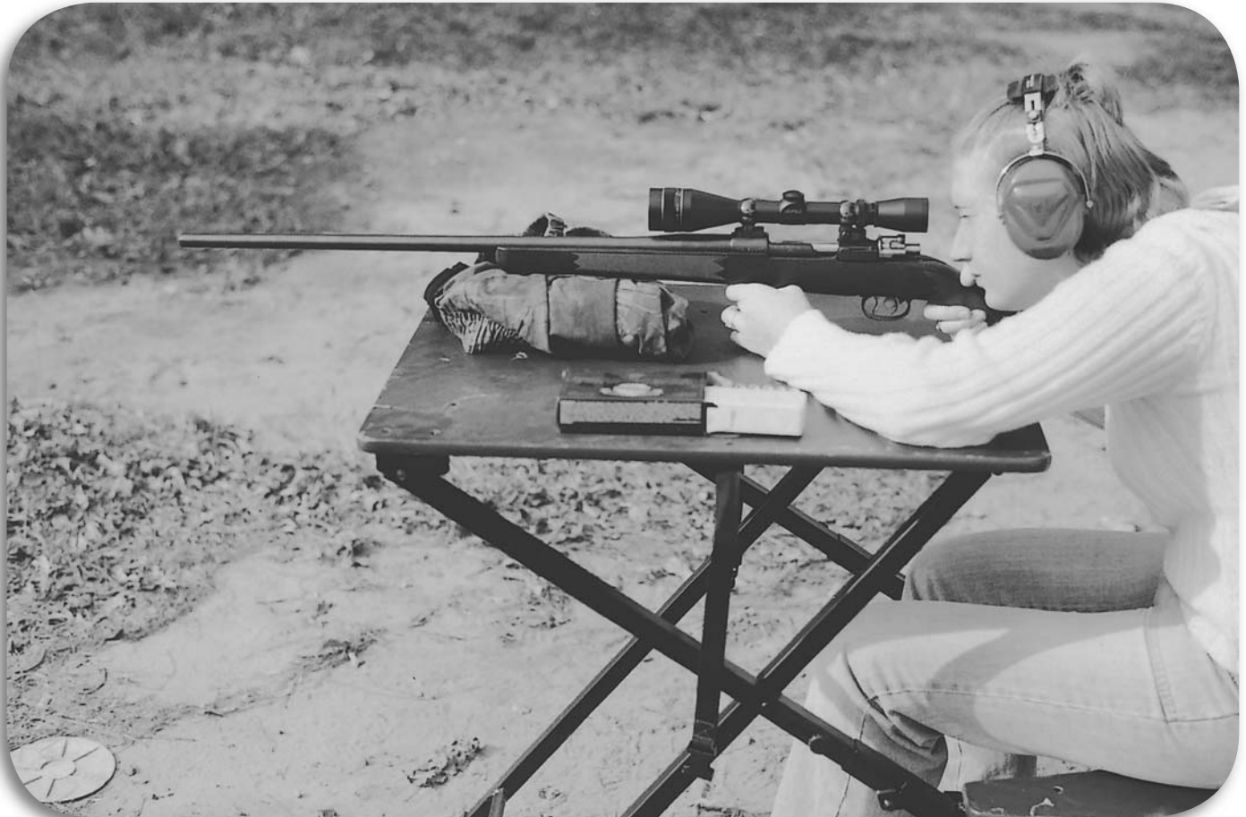
Precision rifles are important combat tools and with good ammunition, extraordinary results can be obtained. This custom rifle carries a Shilen barrel and a Leupold & Stevens scope. It consistently delivers 0.6-inch groups at the 100-yard range.
