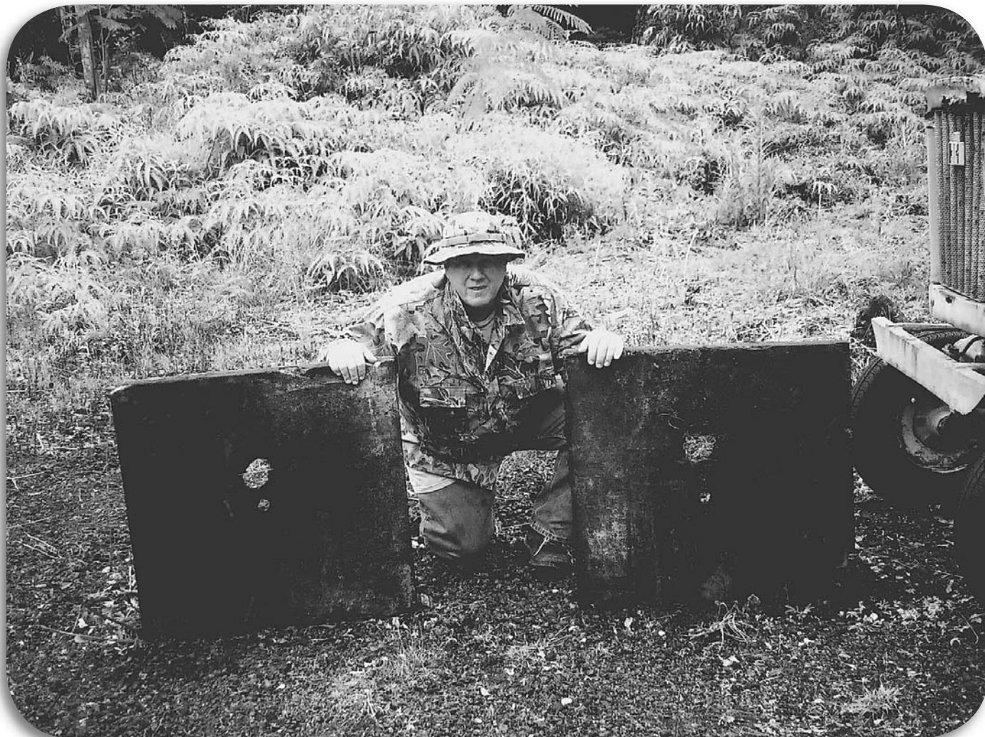
Ace Kaminski poses with the two three-inch concrete blocks that were punctured by the 338 Laupua Magnum loads during test of the rifle.
