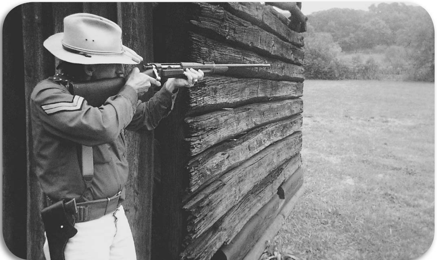
Big bore and full-power do not always work well. This Krag carbine was liked for its light weight, but did not work well with the 220-grain bullet in a full-length rifle.
