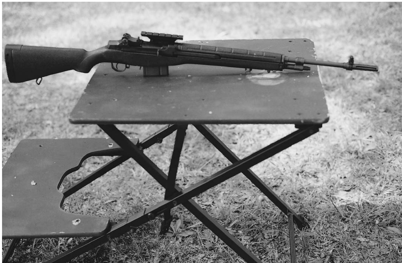
The Springfield Armory clone of the military-built M-14 is marketed with a B-Square scope mount. The rifle's receiver is drilled and tapped to handle the mount.
