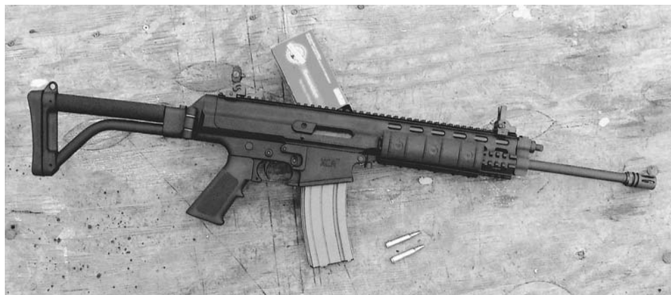
Robinson Armament's XCR rifle brings some new thinking to battle arms design. It is being developed to handle three different calibers with only minor changes.
