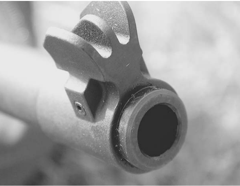
The front sight of the carbine is protected by wings cast with the blade. The current issue of the carbine carries a ghost ring rear sight.
