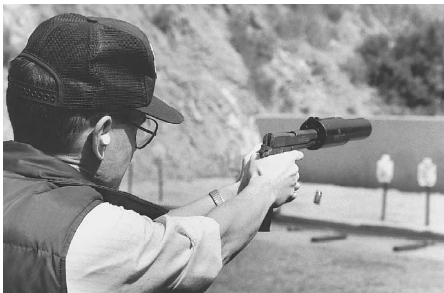
The La France CBB silencer is mounted on a Colt 45 M1911A1 with an extended magazine. Note that the V-type rear sight is a part of the suppressor. This one would be useful in taking out guard dogs and enemy sentries.
