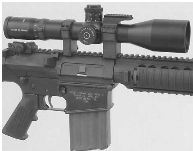
The Mk 11 Mod 0 rifle also carries a Leupold scope, but it is less sophisticated than that now gracing the M110. This scope carries an 8 MOA dot reticle and a standard sunshade.
