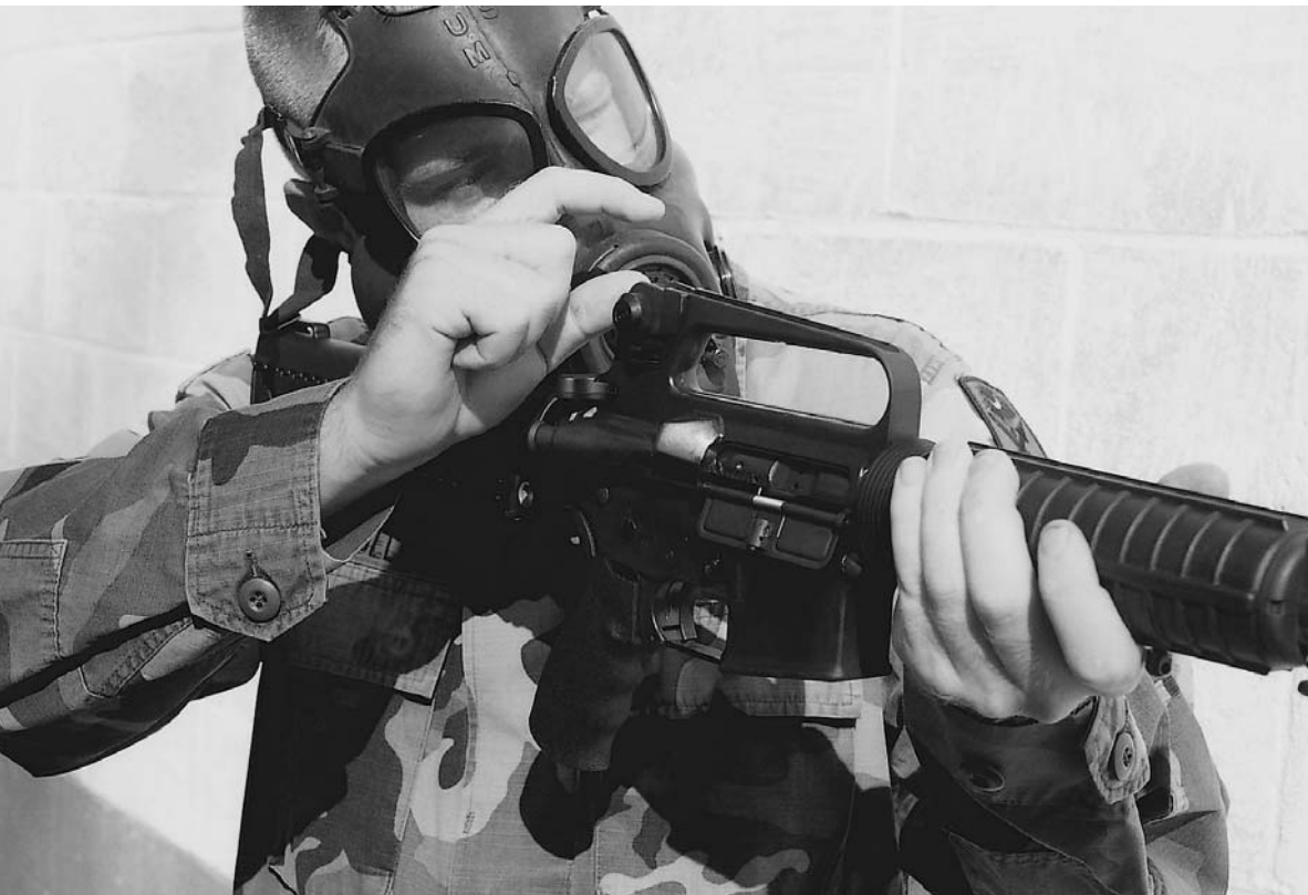
Campbell's soldier son, Matthew, uses his fingers to indicate the increments of adjustment required in firing the AR-15 while wearing a gas mask. Using only the front sight for reference, the rifle tends to fire high.
