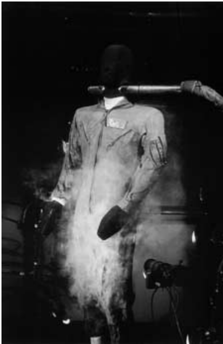
FIGURE 5.7 Nomex® coverall self-extinguishes after torches extinguish.
