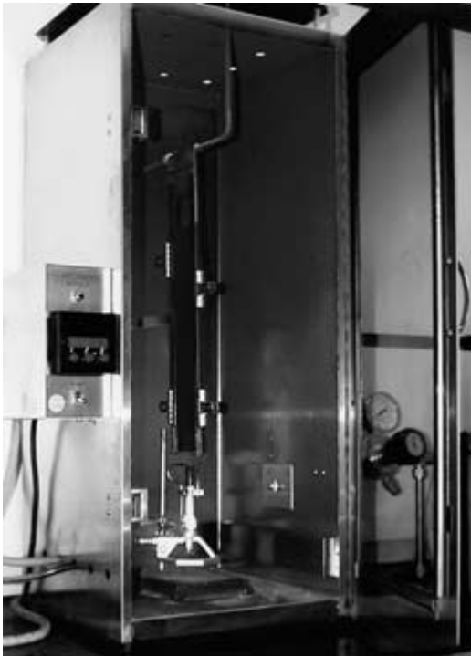
FIGURE 5.1 Vertical flammability test apparatus.
