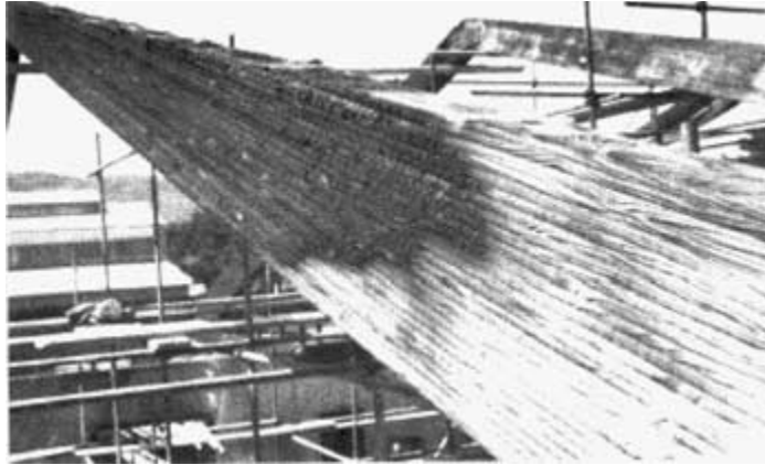
FIGURE 6.21 Wood fire damage 2. (From Ref. 13, p. 275. With permission, John Wiley & Sons, Limited, from Buchanan, Andrew H., Structural Design for Fire Safety , Copyright 2001.)
