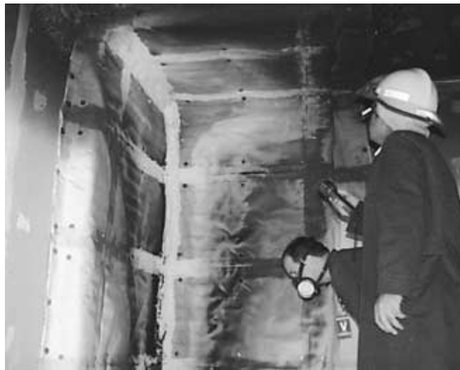
FIGURE 9.20 Composite corner with StructoGard after testing.
