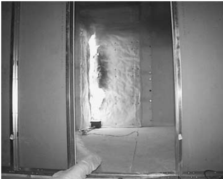
FIGURE 9.16 ISO 9705 fire test during 100-kW fire exposure.
