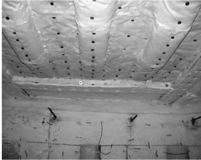
FIGURE 9.31 Solid composite deck panel with fire insulation (Test 4) in the furnace before the fire test.
