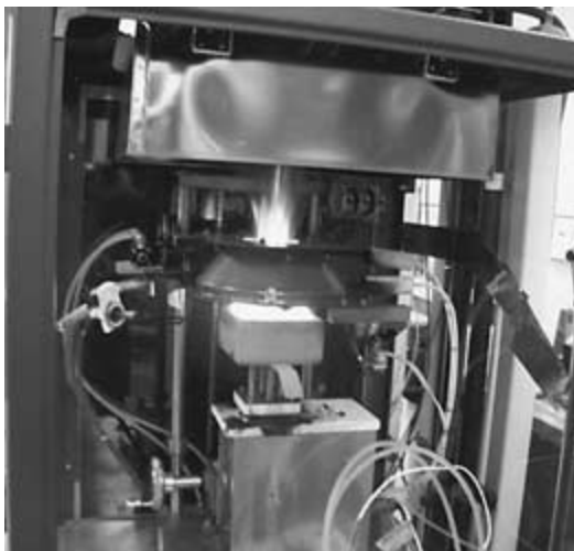
FIGURE 9.12 Cone calorimeter (ASTM E 1354) heat release test.
