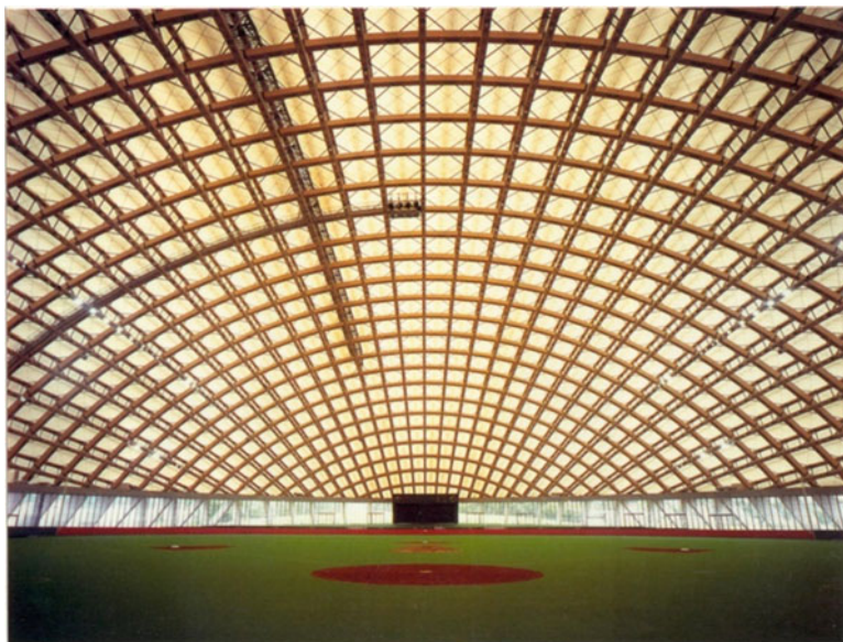
Fig. 8.1 Sports complex in Tver roofed with glulam bearing structures
