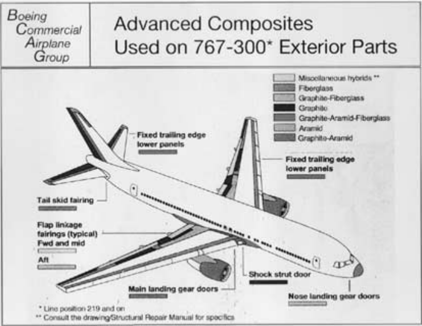
FIGURE 9.5 Use of advanced composite materials in Boeing 767. (D. Baker, AFRL/MLS-OL, Advanced Composites Office, Hill AFB, UT)
