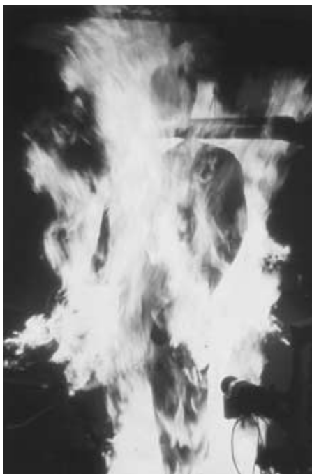
FIGURE 5.5 Flash fire exposure using instrumented thermal mannequin.
