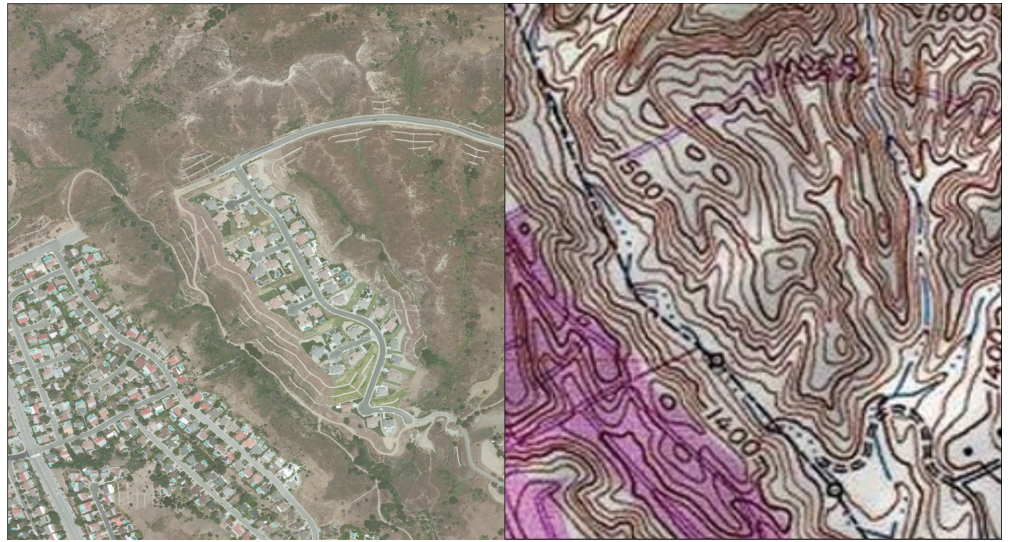
Figure 4.3 Common Raster Graphics Used in GIS Applications: Aerial Photograph (left) and USGS DEM (right)
