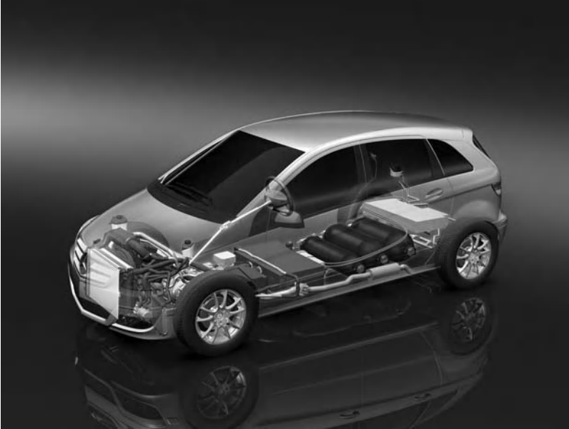
Figure 6.15 Typical \text{CH}_2 tank rack from a European OEM (with kind permission from Daimler AG).
