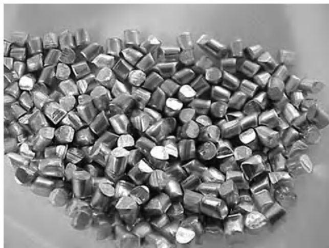
Figure 6.10 Aluminum, recycling of aluminum waste to provide pellets for deoxidation.
