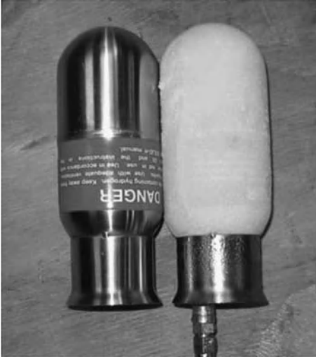
Figure 4.35 The heating and cooling potentials for canisters of metal hydrides (reprinted by permission).
