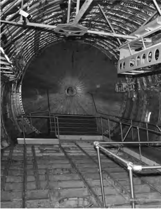
Figure 6.4 Rear pressure bulkhead as an example of a damage-tolerant design (with kind permission from the Auto & Technik Museum Sinsheim e. V).
