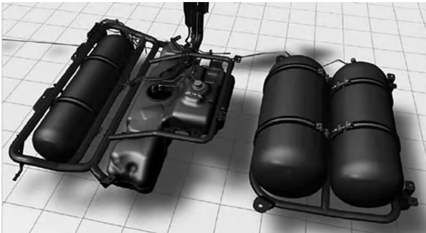
Figure 6.20 Conventional gasoline fuel tank state-of-the art for passenger cars and tank for compressed natural gas.
