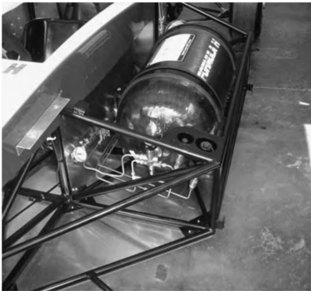
Figure 6.9 Bolted bracket tree on a metal high-pressure pipe.
