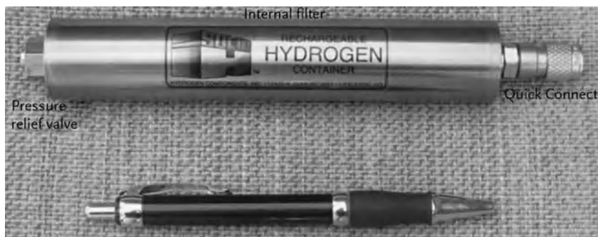
Figure 4.30 SOLID-H model BL-H metal hydride container holds 30 SL of H_2 gas [87], reprinted with permission of Hydrogen Components Inc., Colorado, USA.
