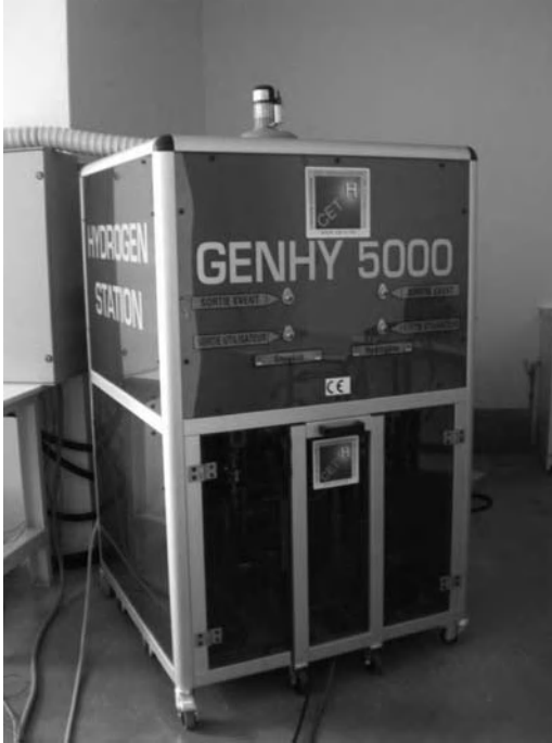
Figure 2.20 GenHy ® 5000 PEM electrolyzer, reprinted by kind permission of P. Millet, Université Paris Sud 11 (UMR 8182) and CETH.
