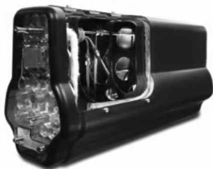
Figure 6.16 Free-form tank design and placement of cryogenic storage tank in the mid-compartment of a BMW vehicle (with permission from BMW Group).
