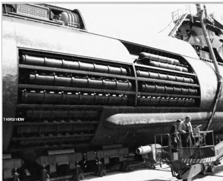
Figure 4.50 Hydrogen storage (based on metal hydride) for supplying hydrogen to Siemens PEM fuel cell [96] (by kind permission of Juergen Giefer, Federal Ministry of Defence, BMVg – Rü VII 3).
