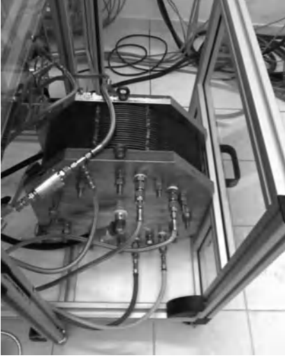
Figure 2.18 GenHy®3000 PEM electrolyzer, reprinted by kind permission of P. Millet, Université Paris Sud 11 (UMR 8182) and CETH.
