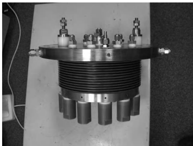
Figure 2.17 GenHy ® 1000 PEM electrolyzer, reprinted by kind permission of P. Millet, Université Paris Sud 11 (UMR 8182) and CETH.
