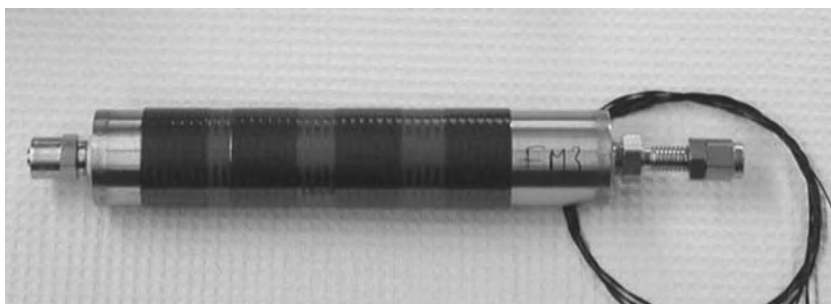
Figure 4.32 Hydrogen container of MASER by SPECTRATIME, reprinted with permission of SPECTRATIME.
