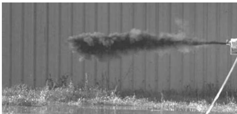
Figure 4.45 Powder expulsion cloud without external source of ignition [55].
