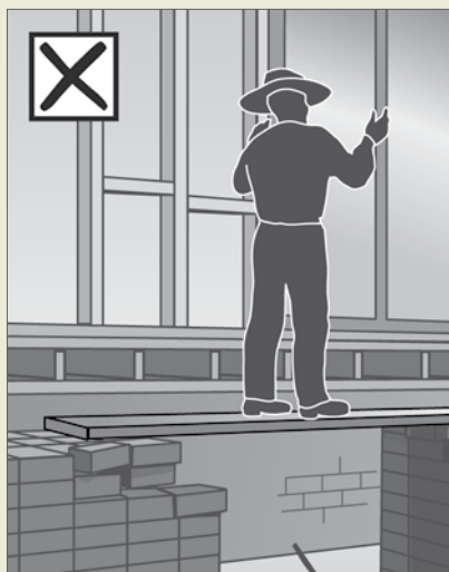
(c) Hazard: makeshift means of gaining height
