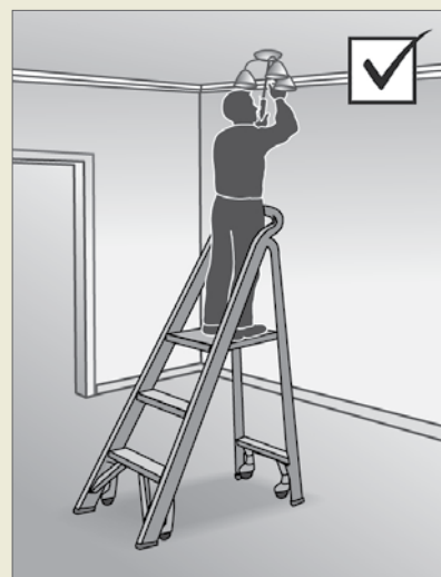
(b) A safer alternative: select the right ladder or step platform for the job
