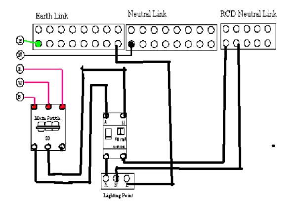
\*Note: Using TPI in conduit, the neutral and earth conductors can be wired directly to the lights and don't need to go through the switches.
