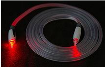
A TOSLINK fiber optic audio cable with red light being shone in one end transmits the light to the other end
