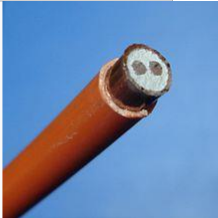
PVC-sheathed MICC cable. Conductor cross section area is 1.5 mm² ; overall diameter is 7.2 mm
