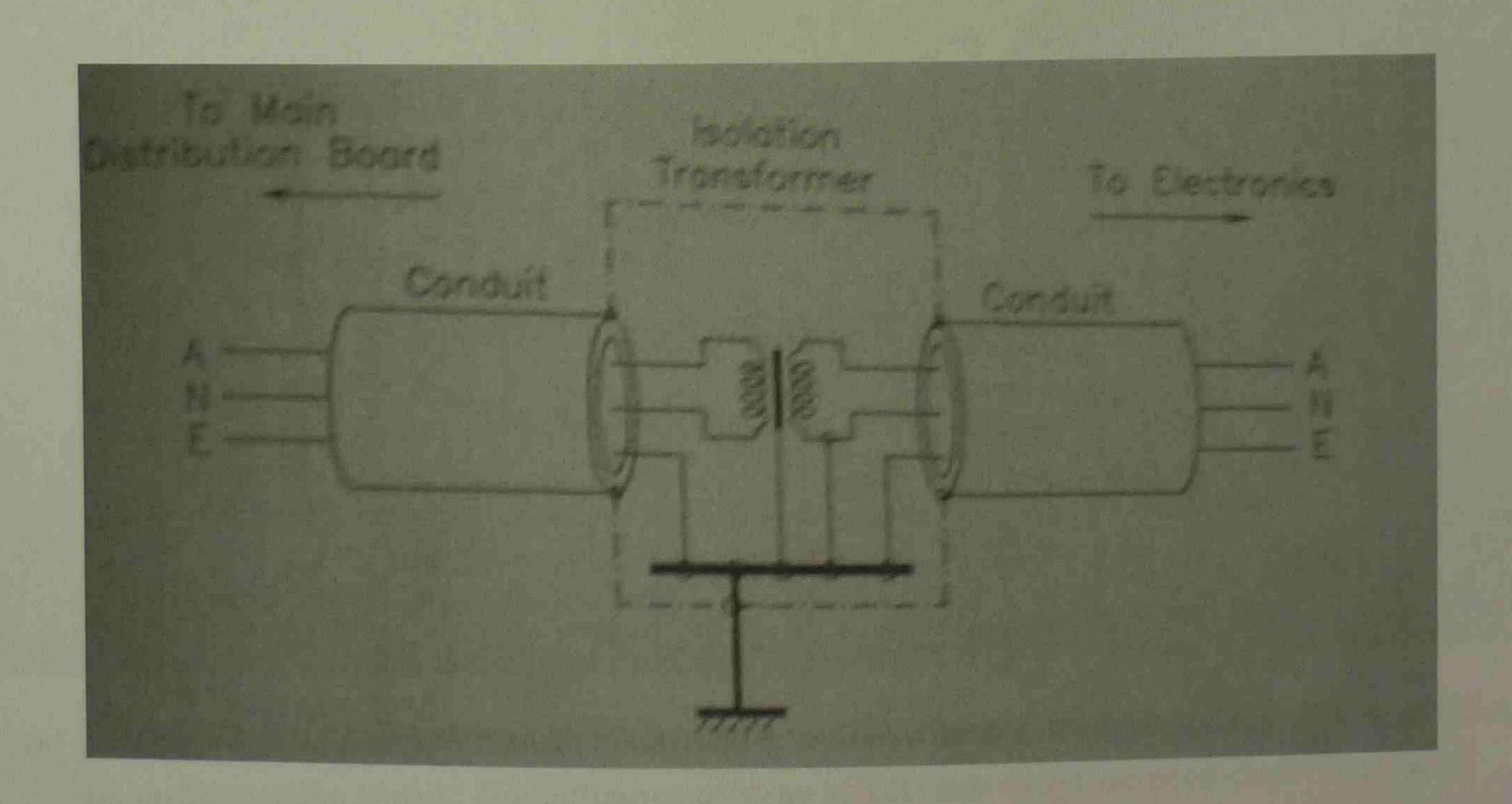
(c) Power Line Conditioners: A Power Line Conditioner is an isolation transformer with some additional feature for regulating the secondary output voltage. The purpose of the voltage regulation is to reduce the effect of voltage surges or dips on the secondary side. These devices are usually used for the power supply to smaller PLC installations.
