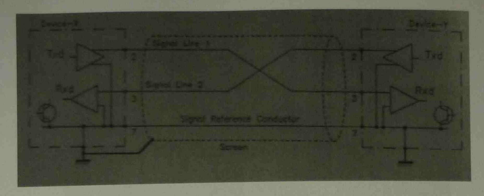
**Screen Earthing:** Signal cables and data communications cables usually include one or more screens, which are not electrically connected to the signal carrying conductors. The method of earthing these screens has a major influence on the noise immunity of the interconnection.
