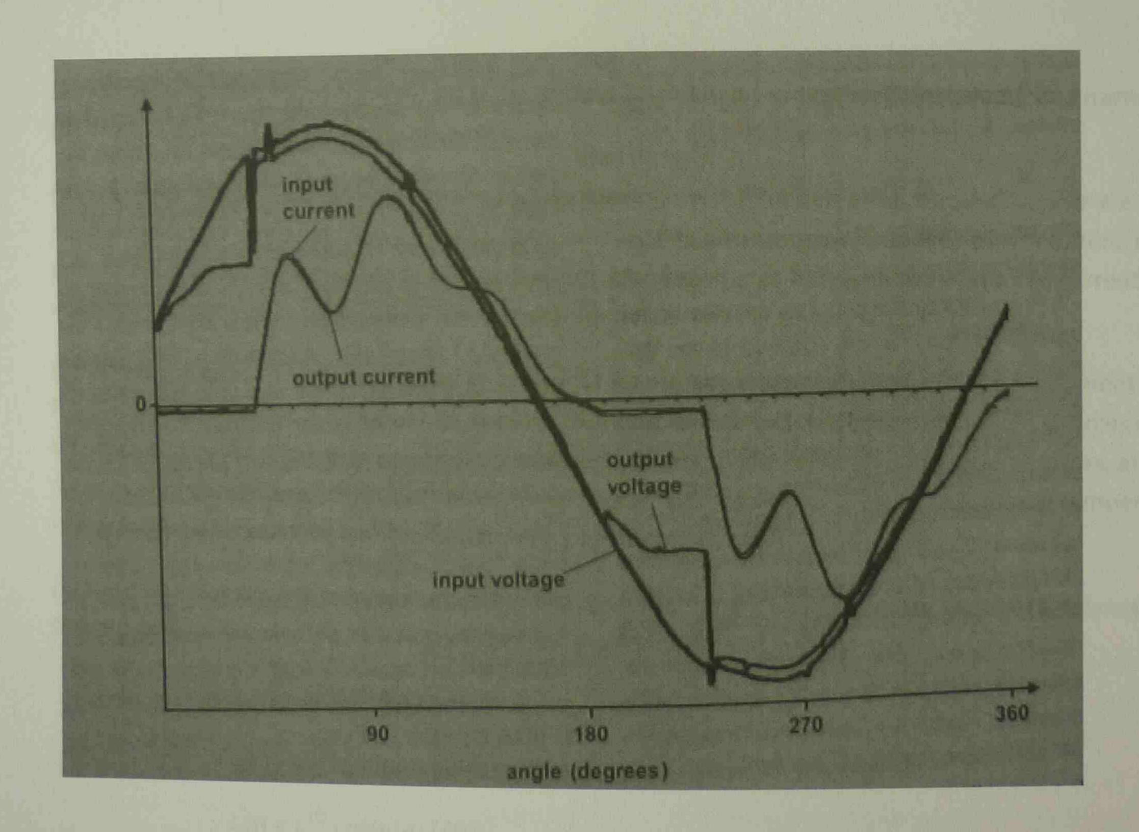
(b) Calculated current of brushless dc motor in full on mode at rated operation.
