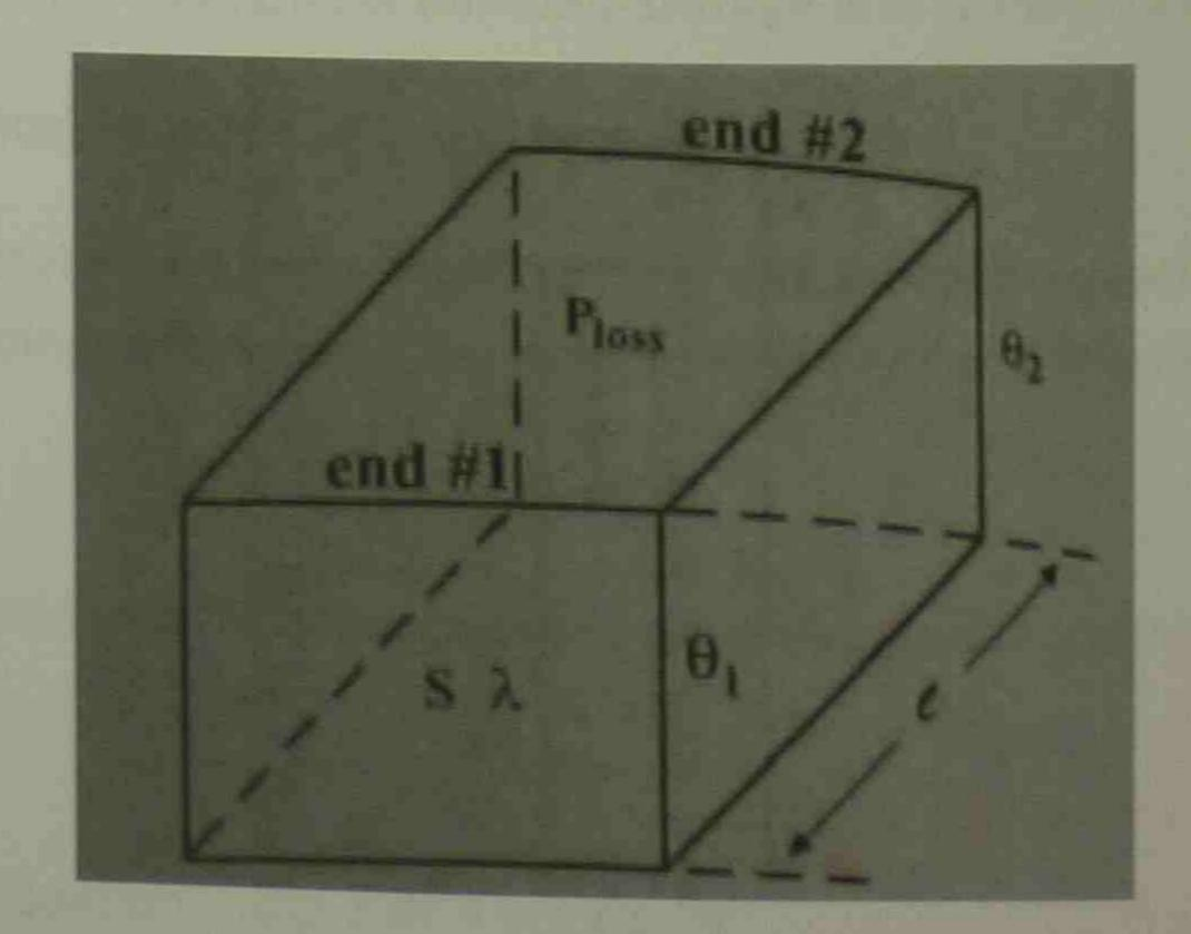
Where  $\lambda$  is the thermal conductivity of a homogeneous body measured in [W/m<sup>0</sup>C], S is the surface of the homogeneous body perpendicular to the heat flow measured in m<sup>2</sup>, and the length of the homogeneous body along the direction of the heat flow measured in m.
