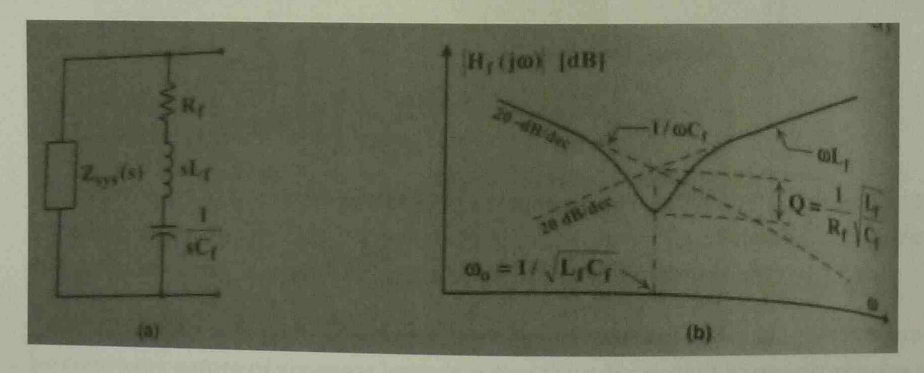
For high-voltage applications, the filter current has a low rms magnitude and does not require large current carrying conductors; therefore, air-core inductors are regularly used and the filter quality factor is relatively large. For low voltage applications, gapped iron-core inductors and conductors with a large cross section are employed.
