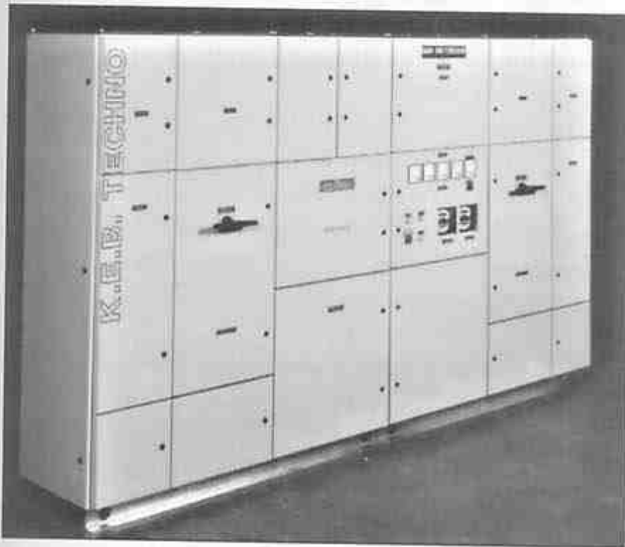
Fig. 17.14 This 2500 A switchboard installed in a flour mill in Papua New Guinea is an example of modular construction. It has been type-tested as complying with AS 3439 K.E. BROWN ELECTRICAL SWITCHBOARDS
