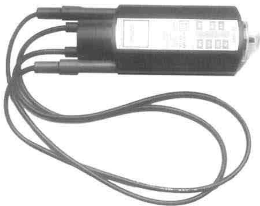
Fig. 11.6 High-impedance tester QUEENSLAND ELECTRICITY COMMISSION
