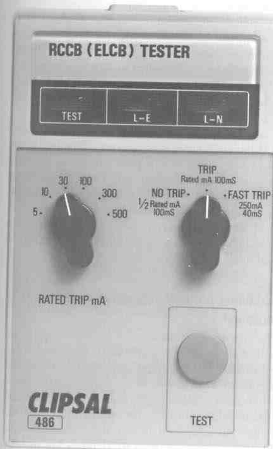
Fig. 14.10 RCD calibration tester GERARD INDUSTRIES
