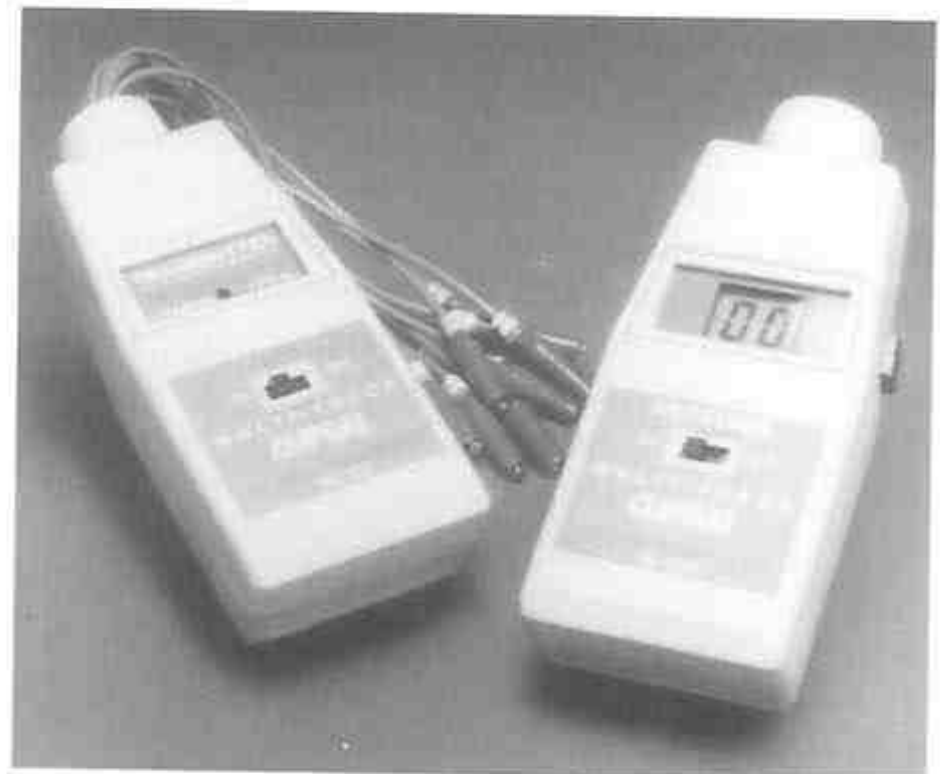
Fig. 11.38 Cable tester for multicable runs GERARD INDUSTRIES
