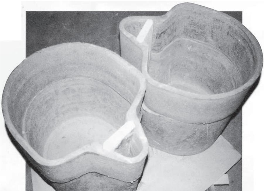
**Figure 11.3** 1100 kg capacity teapot KALTEK ladle.
