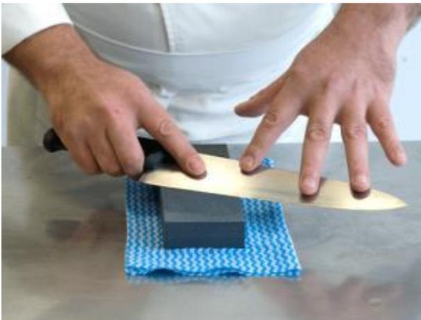
Place knife blade on stone at a 15 degree angle (see below).
