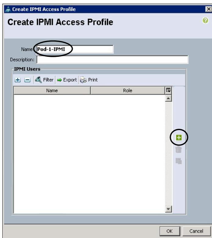
**Figure 18-42** Naming the IPMI Profile
