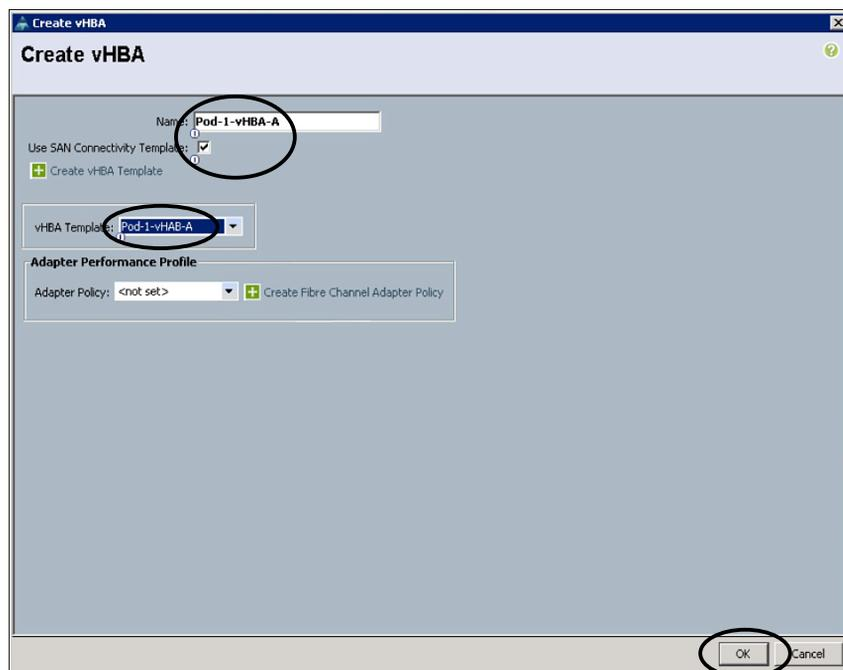
**Figure 18-53** Configuring the Create vHBA Dialog Box While Creating a Service Profile Template
