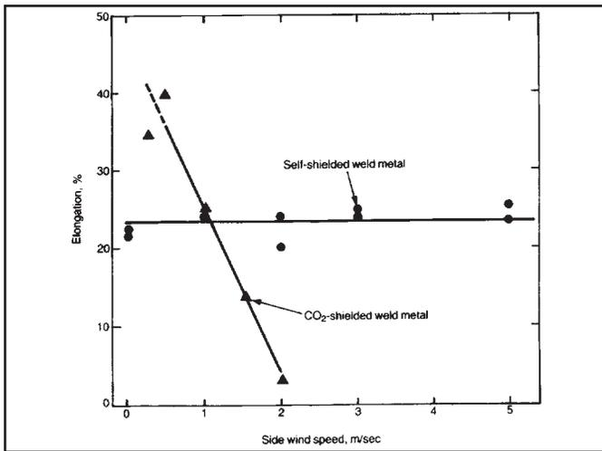
**Figure 3-4a** Comparison of the effect of side wind on tensile elongation of: (a) CO<sub>2</sub>-shielded and (b) self shielded ferritic steel weld metals.
