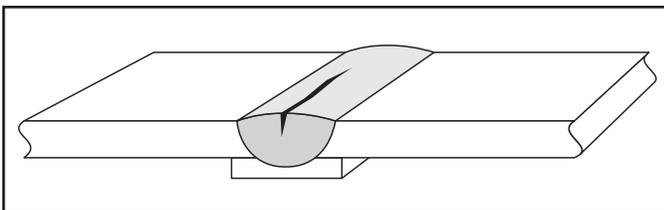
Figure 9-1 Centerline cracking
