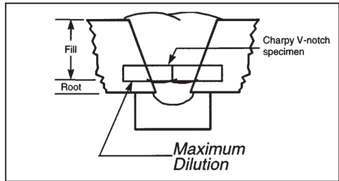
**Figure 6-9** Locations of CVN test specimens
