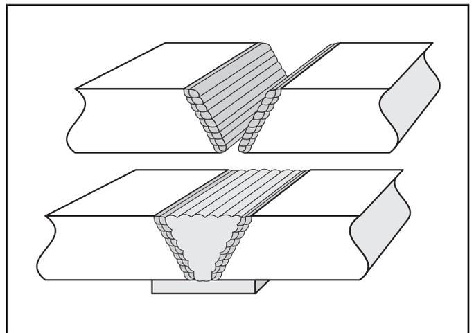
Figure 9-2 Buttering layers
