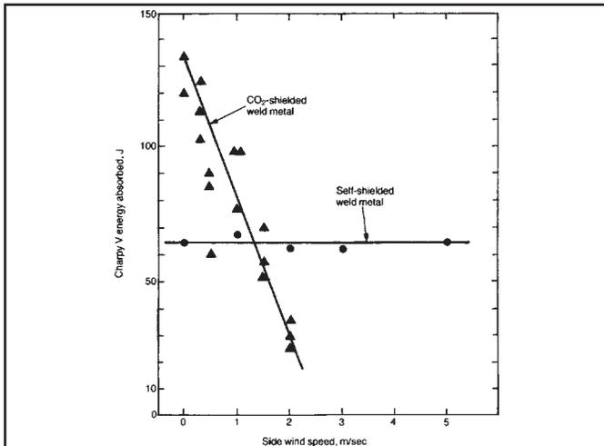
**Figure 3-4b** Comparison of the effect of side wind speed on Charpy V-notch impact toughness of: (a) CO<sub>2</sub>-shielded at room temperature and (b) self shielded ferritic steel weld metals at 0°C.
