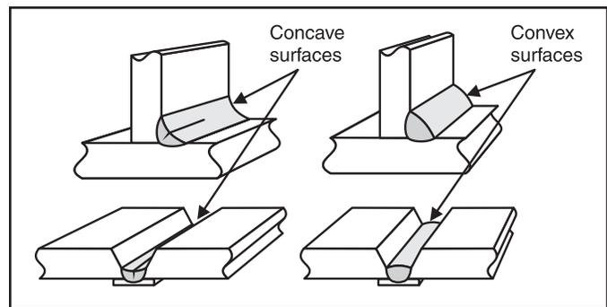
**Figure 9-4** Surface profile induced cracking
