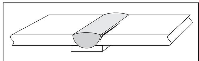
**Figure 9-5** Heat affected zone cracking
