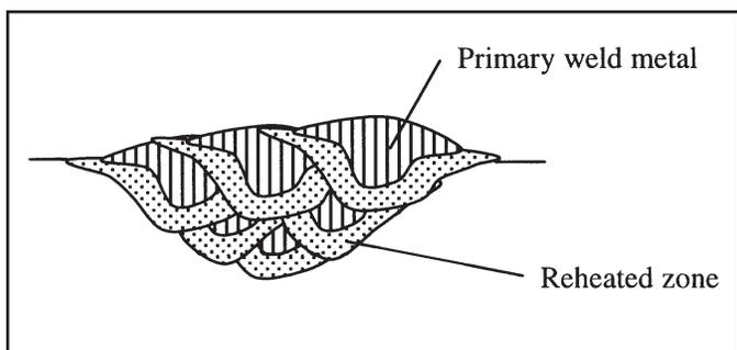
**Figure 6-3** Grain refinement in multiple pass weld
