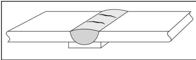
**Figure 9-6** Transverse cracking
