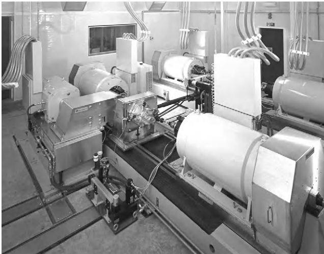
FIGURE 4.13 The five-axis transmission test rig fitted with an electric motor as the engine simulator and a gear-change robot.
