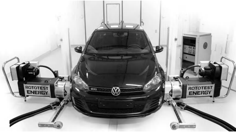
FIGURE 4.12 A “wheel dynamometer” system installed within a garage workshop space having a simple exhaust gas extract system and being used to carry OBD tests. A large cooling fan would be needed in front of the car radiator when running under power. (Photo courtesy of Rototest Ltd.)
