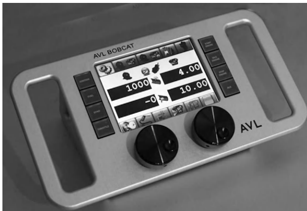
FIGURE 4.11 An example of a portable control pod that can be used both at the main control desk or at an in-cell station during calibration and commissioning. (© AVL NA.)
