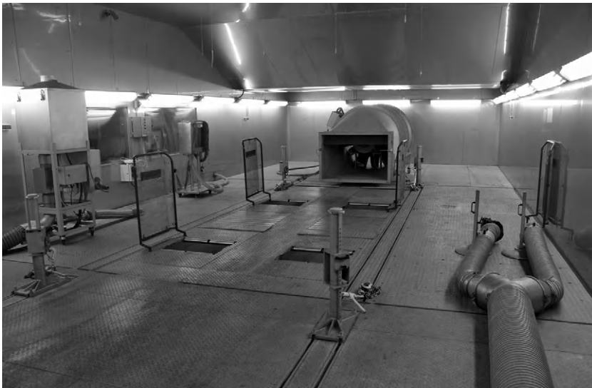
FIGURE 17.5 Climatic cell equipped with 4 \times 4 chassis dynamometer and full exhaust emissions analysis system. All cell surfaces are made from stainless steel. Control room window can just be seen in the left-hand wall beyond the mixing-tee module, which is mounted on castors. Tie-down pillars are in the foreground. Photo by author.
