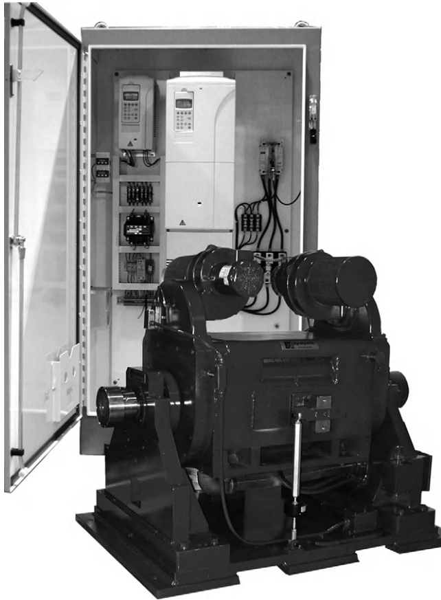
FIGURE 10.3 Typical modern fan-cooled, trunnion-mounted, AC dynamometer and the cabinet housing its power electrics.
