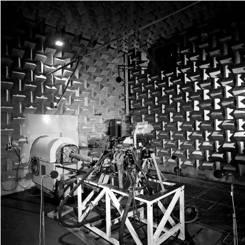
FIGURE 18.1 A semi-anechoic NVH test cell for engine refinement work. Note the two-piece shaft system is connected to a dynamometer installed in the adjoining services room system that includes a pedestal bearing mounted on a plinth, around which are mounted various engine system support and transducer connection boxes. The engine is mounted on a hollow frame and the bedplate mounted on a substantial seismic block. (Photo supplied courtesy of MIRA Ltd.)
