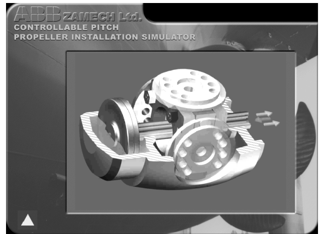
Figure 2: A cutaway view of the Controllable Pitch Propeller.
