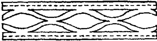
Figure 9.10 Expanded "thermal" girt.
