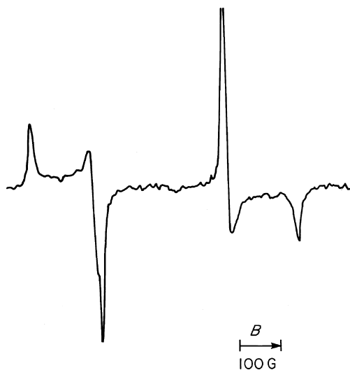
FIGURE 5.11 EPR spectrum of FCO in a CO matrix at 4.2 K. The microwave frequency is 9123.97 MHz. The hyperfine interaction is not quite uniaxial, as is seen by the incipient splitting of the second peak from the left. [After F. J. Adrian, E. L. Cochran, V. A. Bowers, J. Chem. Phys. , 43 , 462 (1965).]
