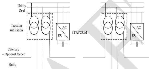
Fig. 5. STATCOM based ERPSS
