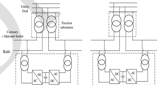
Fig. 6. Railway power conditioner based ERPSS
