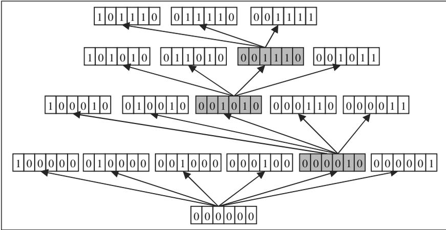
Fig. 8.10 Forward approach for the test case
