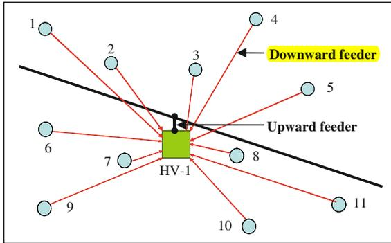
Fig. 7.3 HV substation at a single point
