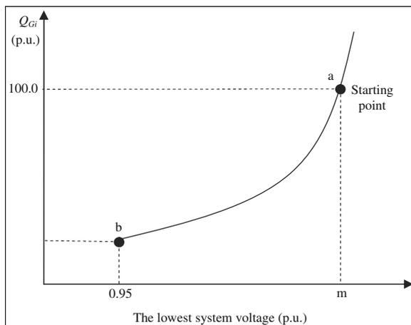
**Fig. 10.7** Step by step procedure for RPC capacity determination
