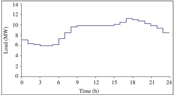
Fig. 4.2 The discretized load of the distribution substation
