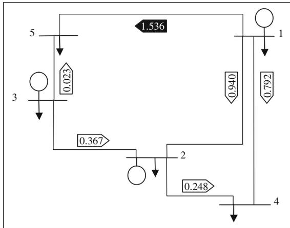
**Fig. 8.4** Flow conditions with 116.5% load increase
