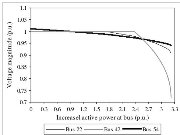
**Fig. 10.6** P–V curves for the modified case
