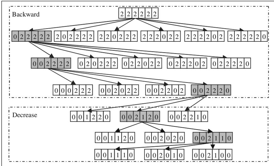
Fig. 8.11 Backward-decrease approach for the test case
