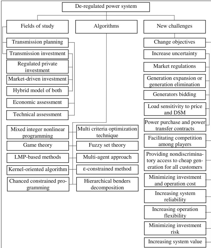
Fig. 12.3 Classification of TEP in de-regulated environment-research trend
