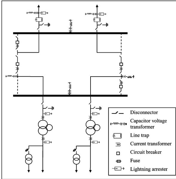
Fig. 1.2 The layout representation of a typical substation
