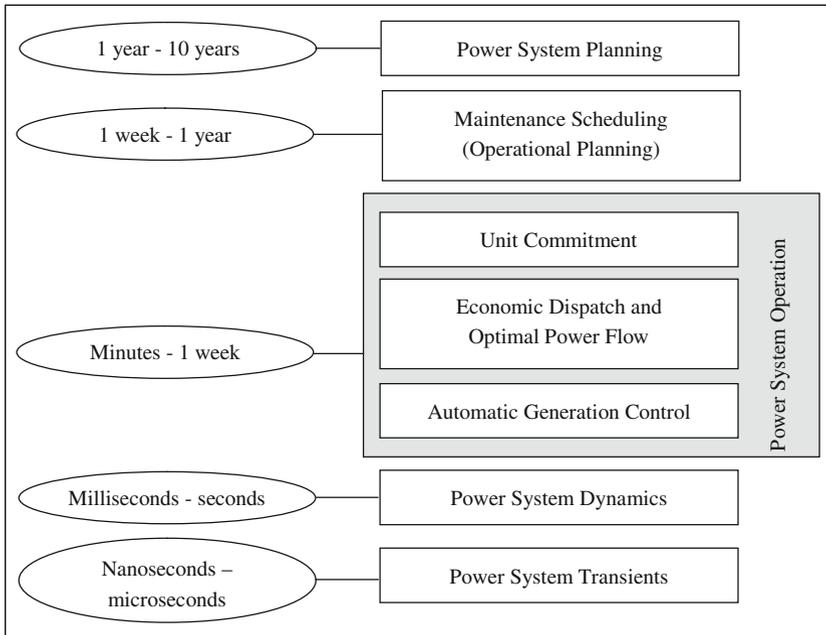
**Fig. 1.3** A time-horizon perspective of power system studies
