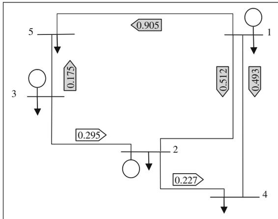
**Fig. 8.3** Flow conditions with 50% load increase
