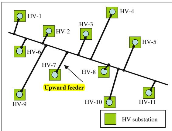
Fig. 7.2 HV substation at each load node
