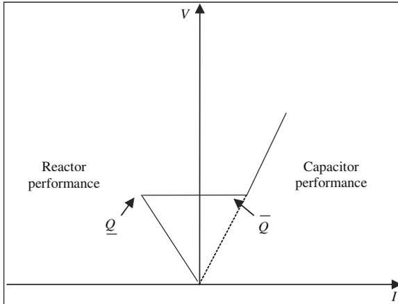
Fig. 10.3 V-I characteristics of an SVC
