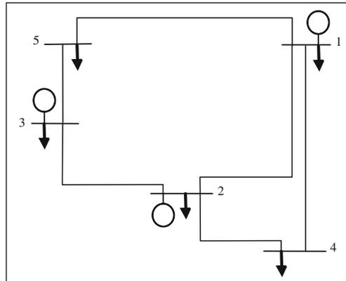
Fig. 6.1 Garver test system
