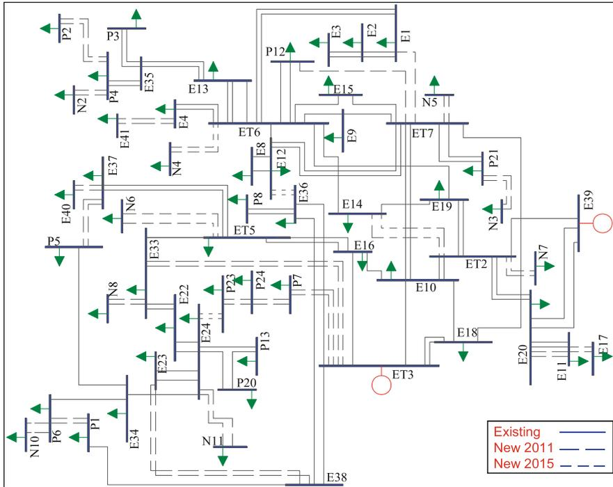
Fig. 13.2 Existing as well as new expansion requirements (63 kV)
