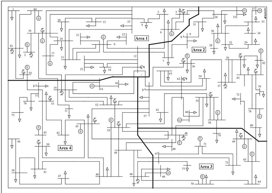
**Fig. 8.13** 84-Bus test system
