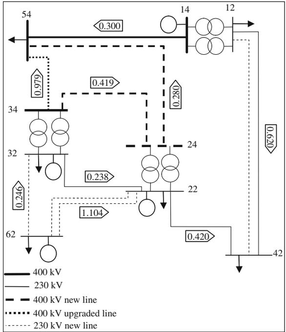
Fig. 9.3 The new test case (scenario 1)
