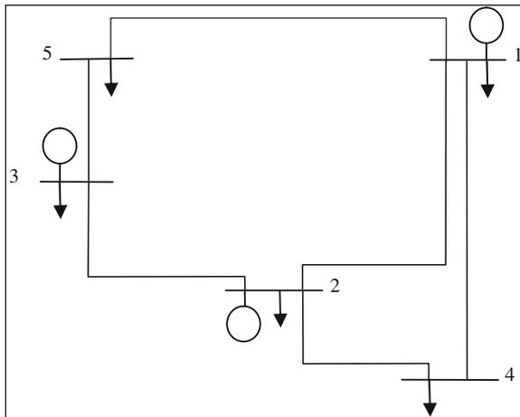
**Fig. F.1** Garver test system
