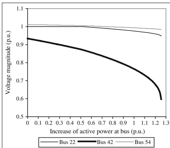
**Fig. 10.5** P-V curves for the base case
