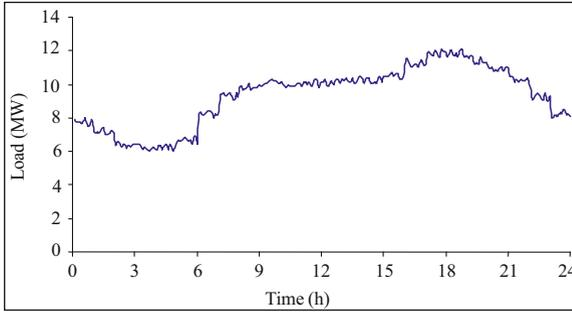
**Fig. 4.1** The daily load of a distribution substation
