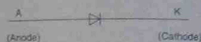
Figure 15.4 • Diode symbol
