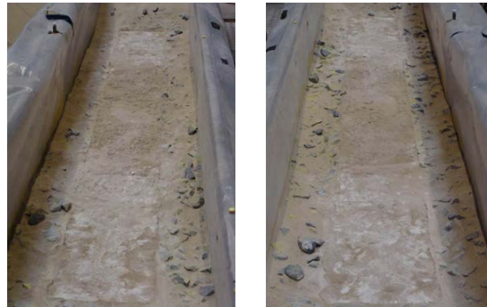
Figure 7.76: Appearance of ballast surface underneath the sleeper after sleeper removal viewed from opposite ends
