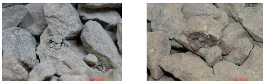
Figure 7.42: Typical ballast particle breakage identified by visual observation
