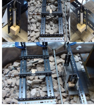
Figure 6.44: LVDTs instrumentation on the sleeper
