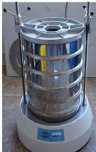
Figure 6.48: Sieves and shaker for PSD test
