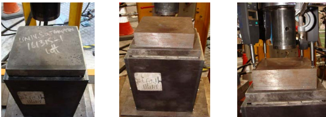
Figure 6.24: The arrangement of ballast sandwich test
