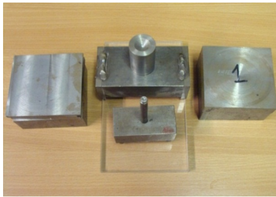
Figure 6.40: The set of known loads and metal rods used for calibration test
