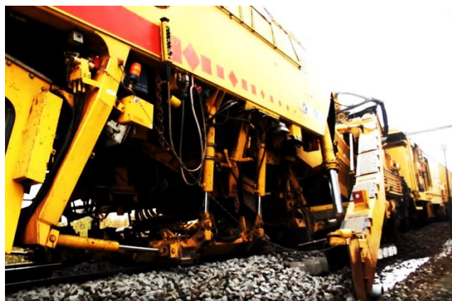
Figure 2.8: The C750 ballast cleaning machine (Courtesy Strukton Rail).
