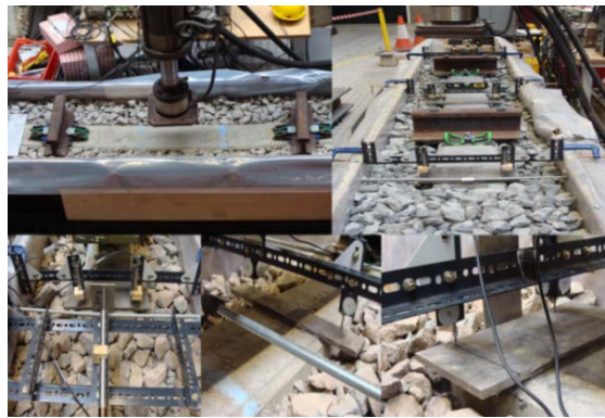
Figure 6.9: The arrangement of the sleeper on the ballast and instrumentation of LVDTs
