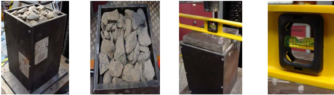
Figure 6.23: Sample preparation for ballast sandwich tests
