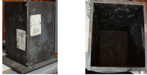
Figure 6.22: The steel square tube used in ballast sandwich test
