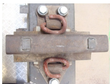
Figure 7.54: A sleeper chair for a proper rail arrangement on plastic and timber sleepers
