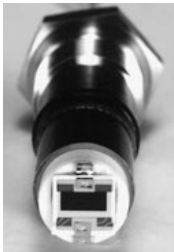
FIGURE 12 Aluminum oxide probe-mounted sensor.
