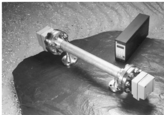
FIGURE 27 Precision water in oil analyzer and cell.
