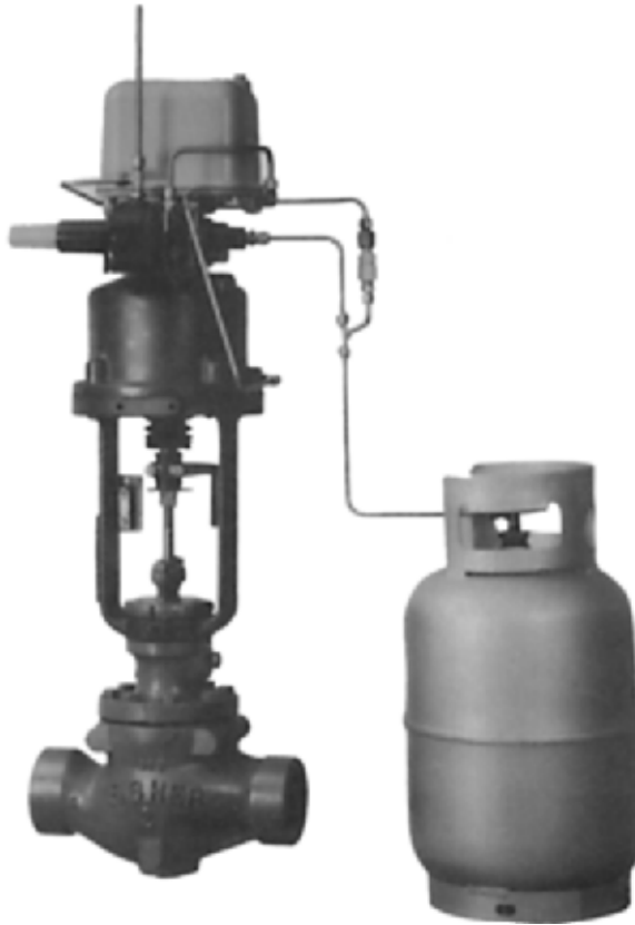
FIGURE 45 Fail action for piston actuators can be accomplished by using pneumatic trip systems. A switching valve transfers stored pressure from volume tanks to the piston to stroke the valve and maintain the predetermined failure position. ( Fisher Controls International, Inc. )
