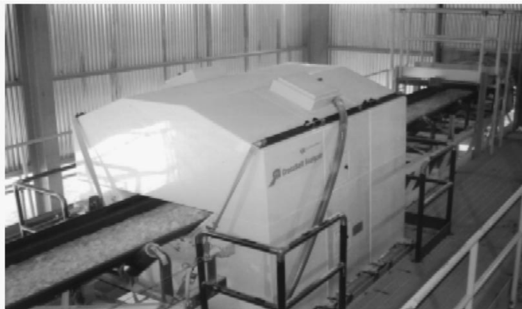
FIGURE 41 Cross-belt analyzer analyzing limestone rock on a 1000-mm trough belt at several hundred tonnes per hour.
