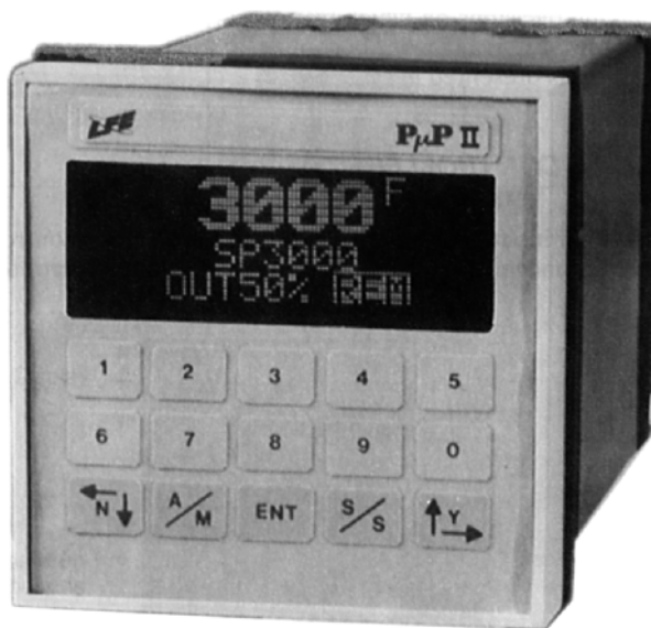
FIGURE 4 Microprocessor-based \frac{1}{4} DIN [96 by 96 mm (3.8 by 3.8 in.)] configurable controller. Instrument features blue vacuum fluorescent dot-matrix display (four lines of 10 characters per line), and self-tuning based on one-shot calculation of the optimum PID values based on a “cold” start. Calculated PID values are stored and can be displayed or changed on demand. Both direct- and reverse-acting outputs can be self-tuned. Four PID settings can be stored for each control output. PID set selection may be programmed as part of a profile, initiated by process variable value, internal trigger, keystroke, or logic input signal. Controller uses a dynamic memory rather than fixed allocation of memory. User can assign memory as needed during configuration for best memory utilization. Security by user ID number can be selected at any program level to prevent unauthorized access and program or data changes. Self-diagnostics are used on start-up and during normal operation by monitoring internal operations and power levels. Upon detection of an out-of-tolerance condition, controller shuts off output(s), activates alarm(s), and displays appropriate message. Controller can perform custom calculations using math programs. Device maintains a history file of event triggers as a diagnostic tool. Two process inputs and four outputs can be assigned to two separate control loops creating a dual-loop controller. Optional features include parallel printer output, logic I/O, digital communications, and PC interface. ( LFE Instruments. )
