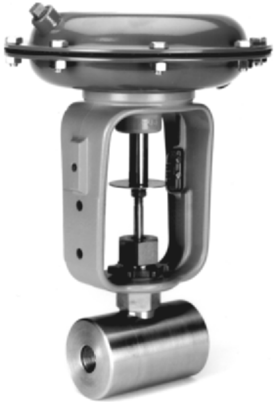
FIGURE 6 Bar-stock valves provide economical solutions to small flow requirements. Pressures to 1500 psig (104 bars) and temperatures to 450°F (232°C) can be handled. Compact spring-and-diaphragm actuators complement these small valve bodies. (H. D. Baumann Inc.)
