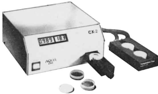
FIGURE 28 Chilled-mirror hygrometer for water activity measurements ( courtesy Decagon Devices, Inc. ). A chilled-mirror hygrometer specifically designed for measurement of water activity. The instrument includes special containers for the substances to be measured. Both dew point and temperature of the vapor immediately above the substance are measured and relative humidity (water activity) is calculated by a microprocessor.
