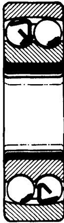
Figure 9.12 Double-row internal self-aligning bearing.
