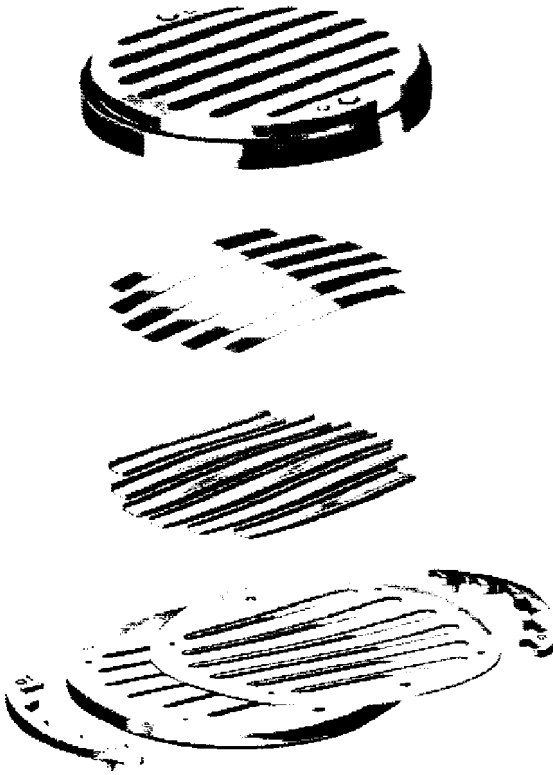
Figure 12.10 Channel valve configuration.
