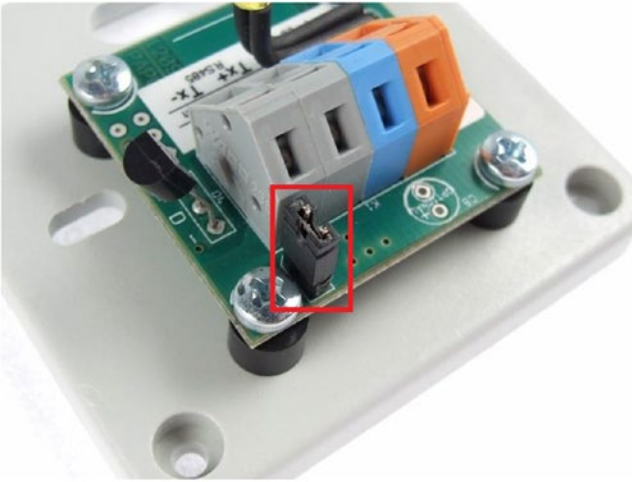
Figure 7-7. Setup jumper is shorted to enable the Modbus RTU. Image courtesy of Papouch ( http://www.papouch.com )
