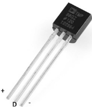
Figure 5-15. TMP36 pin layout
