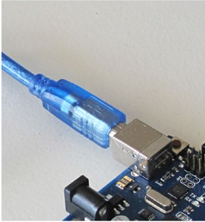
Figure 2-16. USB type A/B cable (type B end) connected to Arduino UNO. Image credited to the “original creator”
