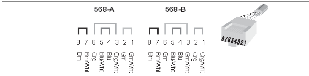
Figure C-2. UTP Wiring
