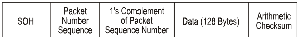
Figure 8.6 Layout of XMODEM protocol
