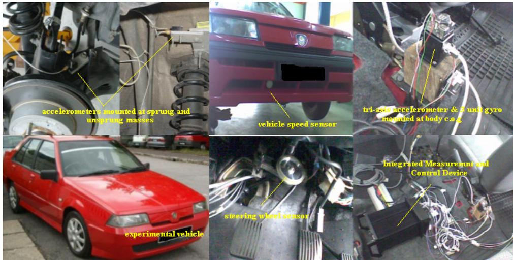
Fig. 5. Instrumented experimental vehicle
