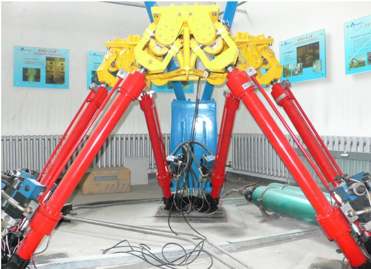
Fig. 4. Experimental hydraulic 6-DOF parallel manipulator
