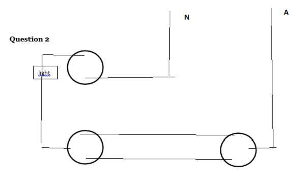
Wire the light with the switches in two way switching
