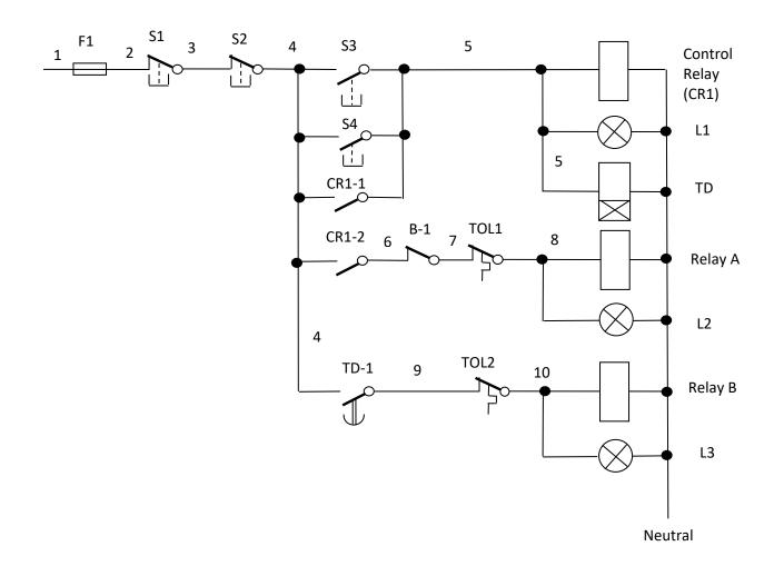
S1/ S2- Magnetic Circuit Breakers Normally Open S1+S2 close----S3 or S4 closes----Control relay CR1 is energised. Lamp L1 indicates it. Then the contact CR1-1 is closed by Control Relay CR1
