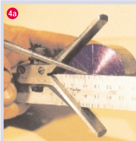
4a A 'centre stock square' is a tool designed specifically for marking centre lines on round objects. This tool is usually bought as part of an engineering combination square set.
