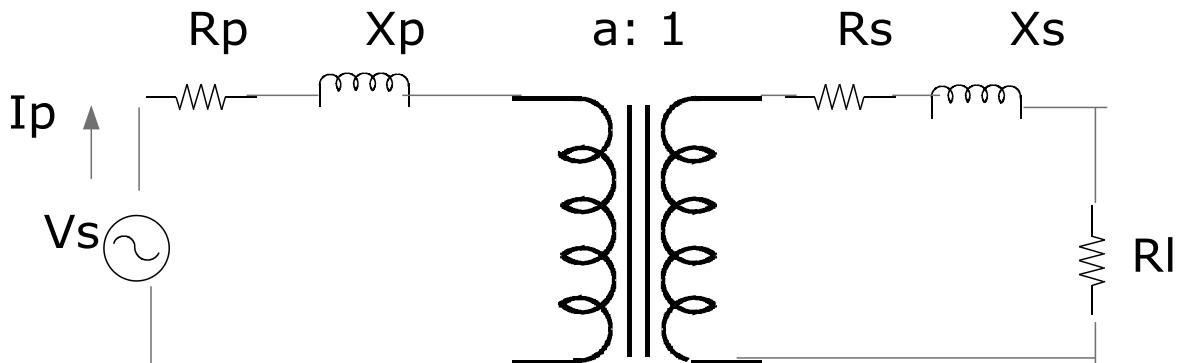
$$I_p = 10 \text{ A}, R_p = 1 \Omega, X_p = 2 \Omega, a = 2, R_s = 1 \Omega, X_s = 2 \Omega, R_I = 50 \Omega$$
