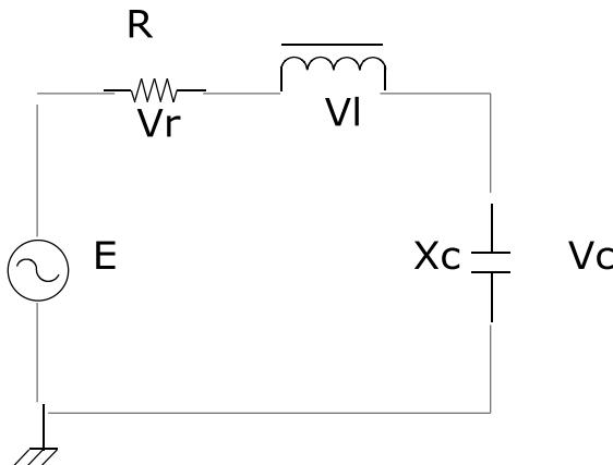
$$E = 10 \angle 0^\circ \text{ V} \quad R = 2 \text{ Ohm}, \quad Xl = 10 \text{ ohm}, \quad Xc = 10 \text{ ohm}$$
