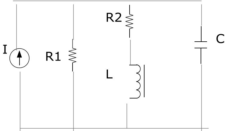
$$R_1 = 40 \text{ k}\Omega, R_2 = 10 \Omega, L = 1\text{mH}, f_p = 0.04\text{MHz}$$
