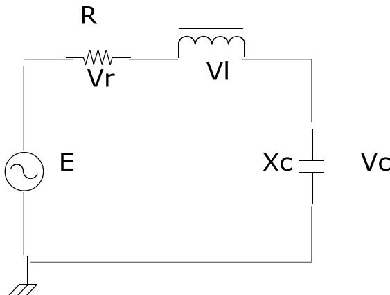
$$E = 10 \angle 0^\circ \text{ V} \quad R = 2 \text{ Ohm}, \quad Xl = 10 \text{ ohm}, \quad Xc = 10 \text{ ohm}$$
