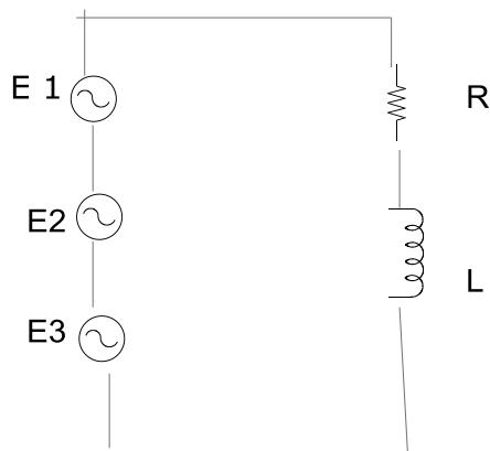
$$E_1 = 25V, E_2 = 80 \sin \omega t, E_3 = 20 \sin 3\omega t, R = 20 \Omega, L = 0.2H$$
