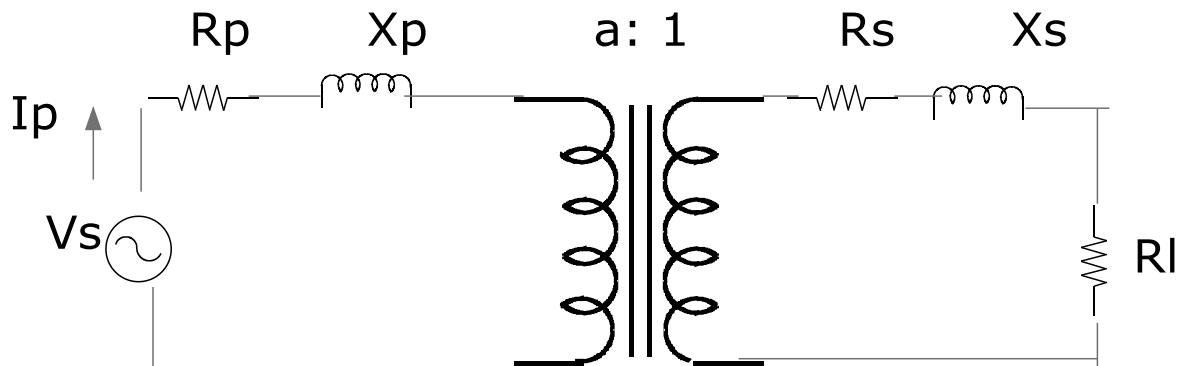
$$I_p = 10 \text{ A}, R_p = 1 \Omega, X_p = 2 \Omega, a = 2, R_s = 1 \Omega, X_s = 2 \Omega, R_I = 50 \Omega$$
