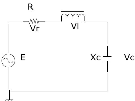
$$R = 2 \text{ ohm}, \quad Xl = 10 \text{ ohm}, \quad Xc = 10 \text{ ohm}, \quad E = 10 \angle 0^\circ \text{ V}$$
