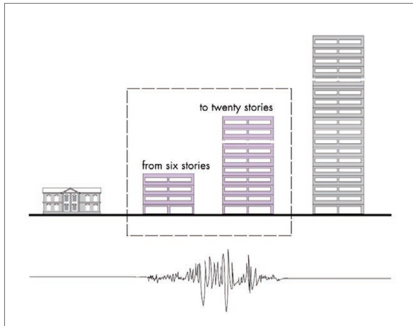
Figure 4-5: The vulnerable group: Mexico City, 1985. The periods of buildings in the 6 to 20 story range resonated with the frequency content of the earthquake.
