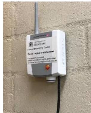
Figure 10 Testo Saveris 1 - T3D data logger.
