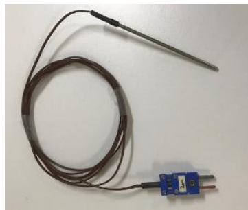
Figure 8 Temperature probe with mini connector.
