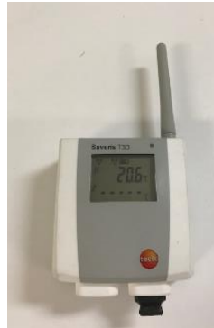
Figure 10 Testo Saveris 1 - T3D data logger.
