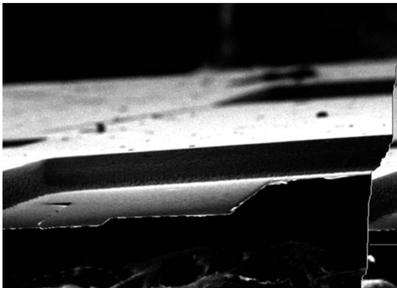
FIGURE 22.22 SEM photo of the 2\mu\text{m} thin GaAs/AlGaAs membrane and of the selective dry etching profile.
