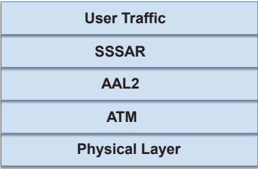
Figure 7.32 A3 interface protocol architecture (user data). SSSAR, Service Specific Segmentation and Reassembly; AAL2, ATM Adaptation Layer 2. Reprinted from Reference [172]. This content, from the TIA-2001-C, “Interoperability Specification (IOS) for cdma2000® Access Network Interfaces Release C,” is reproduced under written permission from Telecommunications Industry Association ( www.tiaonline.org ). All standards are subject to revision, and parties to agreements based on any Standard are encouraged to investigate the possibility of applying the most recent editions of the standards published by them.
