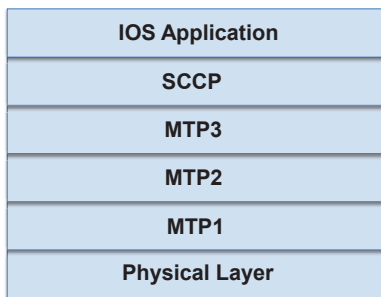
Figure 7.34 A1 protocol architecture (signaling). SCCP, Signaling Connection Control Part; MTP, Message Transfer Part. Reprinted from Reference [172]. This content, from the TIA-2001-C, “Interoperability Specification (IOS) for cdma2000® Access Network Interfaces Release C,” is reproduced under written permission from Telecommunications Industry Association ( www.tiaonline.org ). All standards are subject to revision, and parties to agreements based on any Standard are encouraged to investigate the possibility of applying the most recent editions of the standards published by them.
