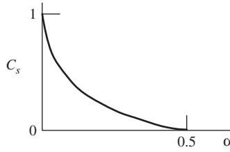
Figure 3.6 Capacity of the binary symmetric channel (BSC) as a function of the channel transition error probability \alpha .
