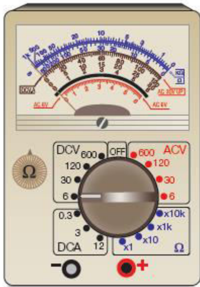
analog multimeter set to read voltage
