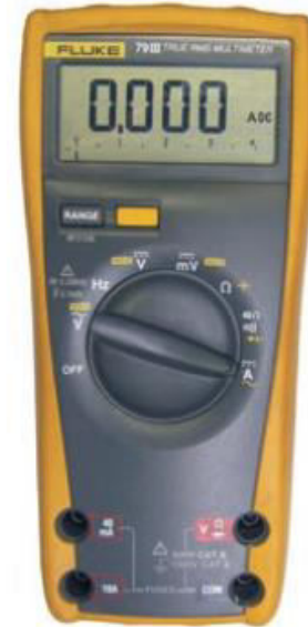
digital multimeter set to read current
