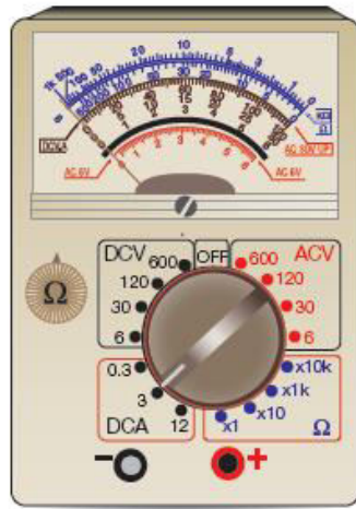
analog multimeter set to read current
