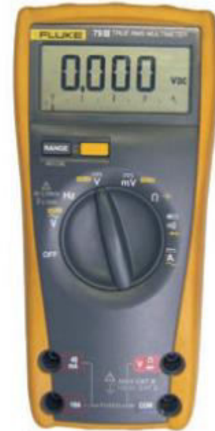
digital multimeter set to read voltage
