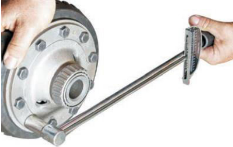
(a) torque wrench with scale indicating the torque being applied to the bolt
