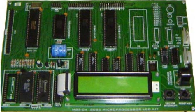
**M85-04** is a single board Microprocessor Trainer Kit based on 8085 Microprocessor, which is widely used to train engineers to develop software/hardware for any industrial process & control. This Kit consists of power-full Monitor EPROM, RAM, I/O Lines, Timer/Counter, Serial, Seven Segment Display and Keyboard for Man to Machine Interface.
