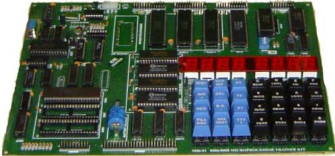
**M86-01** is a single board Microprocessor Trainer Kit based on 16 bit 8086 Microprocessor, which is widely used to train engineers to develop software/hardware for any industrial process & control. This Kit consists of power-full Monitor EPROM, RAM, I/O Lines, Timer/Counter, Serial, Seven Segment Display and Keyboard for Man to Machine Interface.
