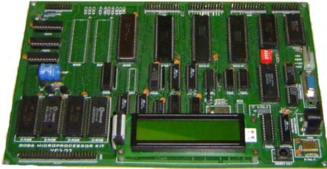
**M86-02** is a single board Microprocessor Trainer Kit based on 16 bit 8086 Microprocessor, which is widely used to train engineers to develop software/hardware for any industrial process & control. This Kit consists of power-full Monitor EPROM, RAM, I/O Lines, Timer/Counter, LCD Display and Keyboard for Man to Machine Interface.
