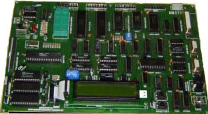
**M85-07** is a single board Microprocessor Trainer Kit based on 8085 Microprocessor, which is widely used to train engineers to develop software/hardware for any industrial process & control. This Kit consists of power-full Monitor EPROM, RAM, I/O Lines, Timer/Counter, Serial, 16x1 LCD Display and Keyboard for Man to Machine Interface.
