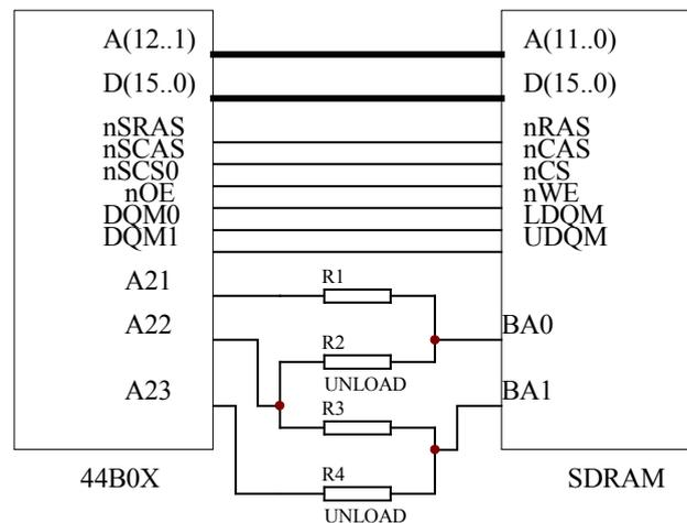
*In the diagram, only two resistances should be uses:*
