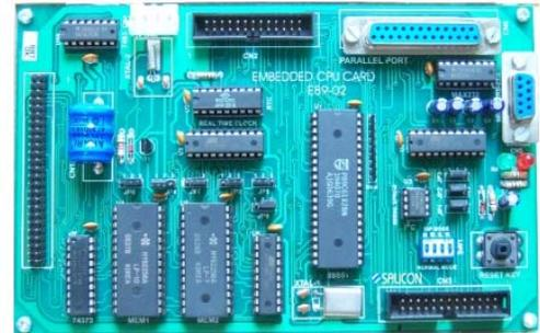
**E89-02** is a single board Embedded Kit based on Philips 8051 Microcontroller for any Embedded applications.
