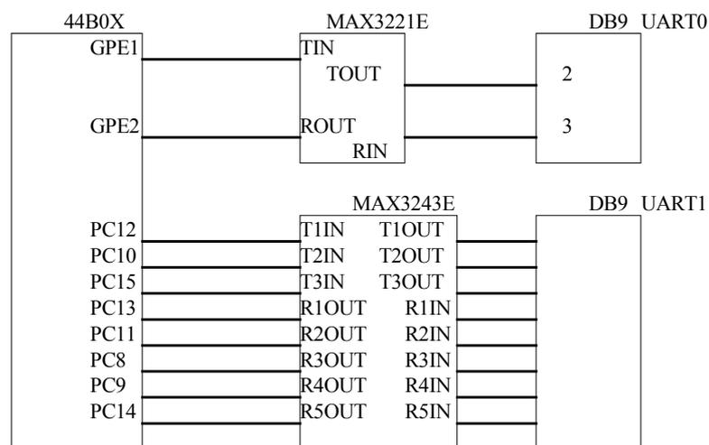
Figure 3-6 Serial Circuit
