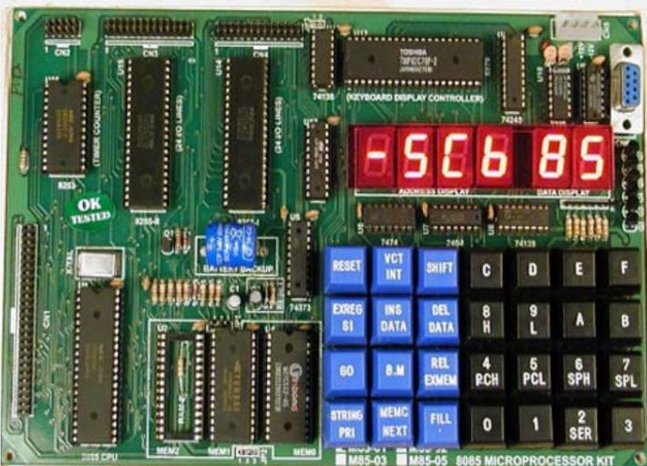
**M85-05** is a single board Microprocessor Trainer Kit based on 8085 Microprocessor, which is widely used to train engineers to develop software/hardware for any industrial process & control. This Kit consists of power-full Monitor EPROM, RAM, I/O Lines, Timer/Counter, Serial, Seven Segment Display and Keyboard for Man to Machine Interface.
