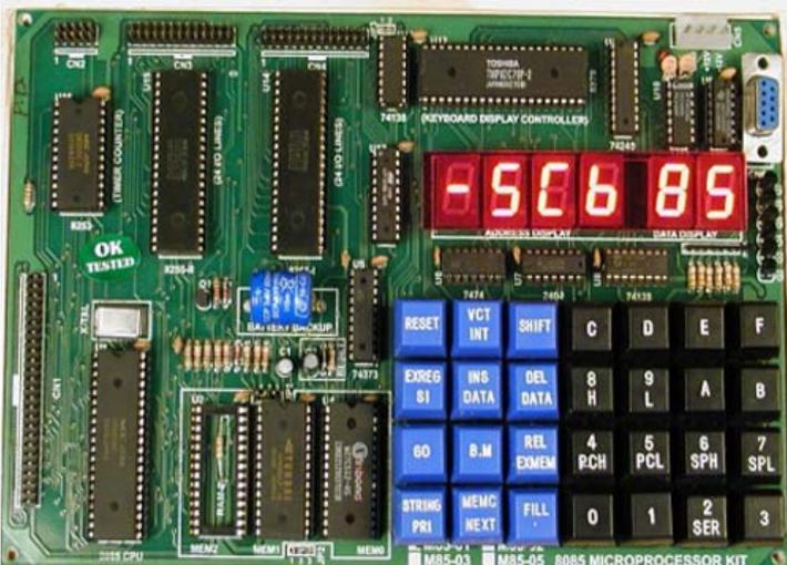
**M85-03** is a single board Microprocessor Trainer Kit based on 8085 Microprocessor, which is widely used to train engineers to develop software/hardware for any industrial process & control. This Kit consists of power-full Monitor EPROM, RAM, I/O Lines, Timer/Counter, Serial, Seven Segment Display and Keyboard for Man to Machine Interface.
