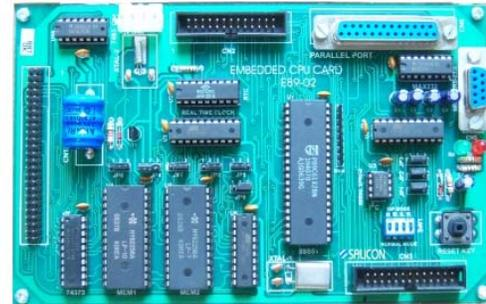
**E89-02** is a single board Embedded Kit based on Philips 8051 Microcontroller for any Embedded applications.
