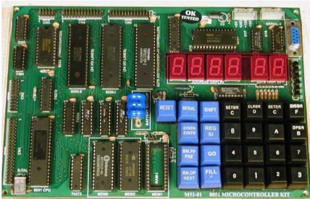
**M51-01** is a single board Microcontroller Trainer Kit based on 8 bit 8051 Microcontroller, which is widely used to train engineers to develop on software/hardware for any industrial process & control. Kit has power-full Monitor EPROM, RAM, I/O Lines, Timer/Counter, Serial, Seven Segment Display, Keyboard for Man to Machine Interface.
