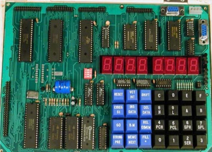
**M85-06** is a single board Microprocessor Trainer Kit based on 8085 Microprocessor, which is widely used to train engineers to develop software/hardware for any industrial process & control. This Kit consists of power-full Monitor EPROM, RAM, I/O Lines, Timer/Counter, Serial, Seven Segment Display and Keyboard for Man to Machine Interface.
