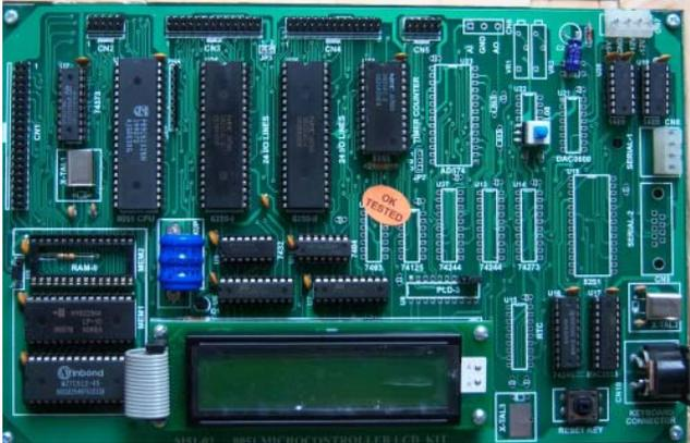
**M51-02** is a single board Microcontroller Trainer Kit based on 8 bit 8051 Microcontroller, which is widely used to train engineers to develop on software/hardware for any industrial process & control. Kit has power-full Monitor EPROM, RAM, I/O Lines, Timer/Counter, Serial, LCD Display, Keyboard for Man to Machine Interface.
