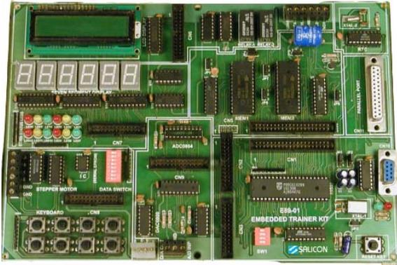
**E89-01** is a single board Microcontroller Trainer Kit based on 8 bit 8051 Microcontroller, which is widely used to train engineers to develop on software/hardware for any industrial process & control.
