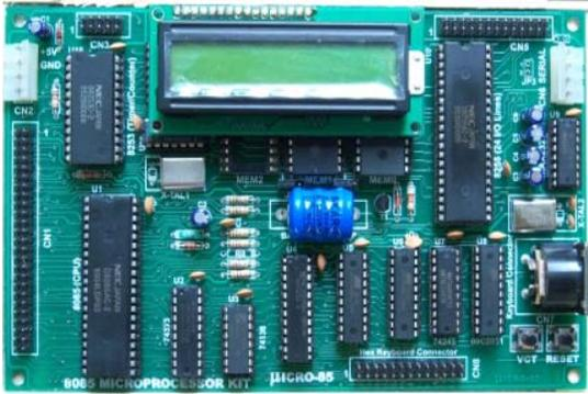
**MICRO-85** is a single board Microprocessor Trainer Kit based on 8085 Microprocessor, which is widely used to train engineers to develop software/hardware for any industrial process & control. This Kit consists of power-full Monitor EPROM, RAM, I/O Lines, Timer/Counter, Serial, 16x1 LCD Display and Keyboard for Man to Machine Interface.
