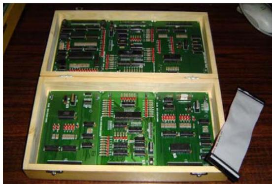
**SC-XX Series** Study Cards can be connected to the 50 Pins KXT Bus of any 8/16 bit Series Microprocessor Trainer Kits. In this Study Card LED's are provided for different signals like Read, Write, Address Lines, Data Lines, Chip Select & Ports depending upon the Peripherals. Study card are supplied in Australian Pine Wood Enclosure.
