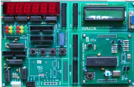
**E89-03** is a single board Embedded Kit based on PHILIPS Microcontroller & PIC Microchip Microcontroller for any Embedded applications
