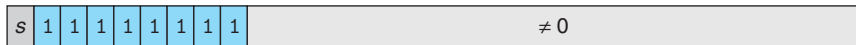
Figure 2.32 Categories of single-precision, floating-point values. The value of the exponent determines whether the number is (1) normalized, (2) denormalized, or a (3) special value.
