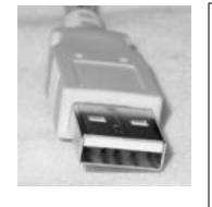
Initially USB version 1.1 supported (2) speeds 1.5 Mb/s and 12 Mb/s. The newest version, ver 2.0 supports up to 480 Mb/s. Up to 127 USB devices can be connected using hubs.
