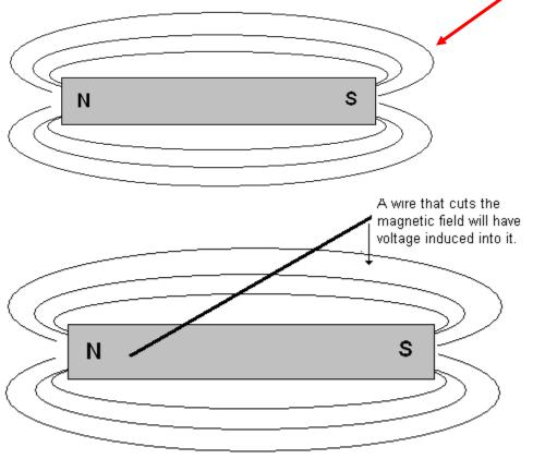
As a piece of wire moves toward the magnet causing it to cut through the invisible magnetic lines, a current is induced into the wire.
