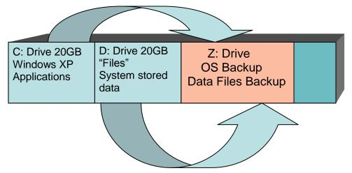
Fig 12.4 Using a single drive to backup the C: Partition and the D: partition
