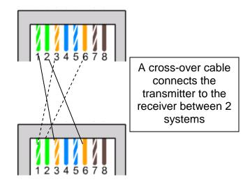
Using a cross-over cable between two systems is an easy way to set up a very small network, but there are no provisions to add any additional computers. A simple solution to this problem is to use a hub to connect computers.
