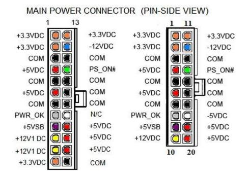
In order to support new systems increasing power requirements, the 20-pin connector has been replaced by a 24-pin connector.
