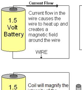
By connecting a wire to each end of a battery, you create a circuit which causes current to flow in the wire. You can't see current flow or the magnetic field around the wire, but you could easily detect the heat being generated.
