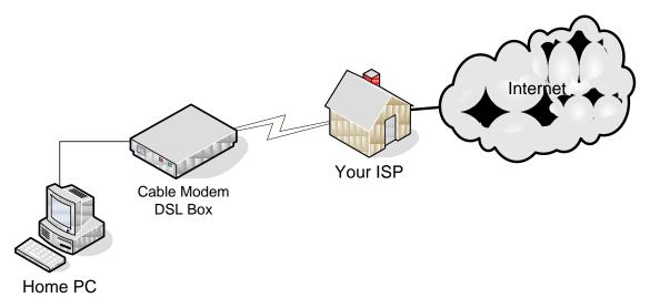
Typical home user Internet Connection using either Cable Modem, or DSL Box
