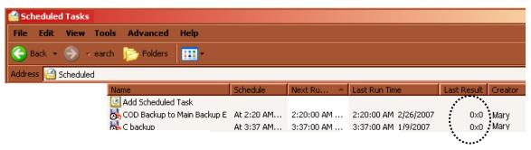
The **Scheduled Tasks** windows shows information about any scheduled tasks. Under the column **Last Result**, if it displays "**0X0**" for the task that indicates that the task ran without an error.
