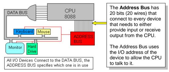
All devices that need to provide input, or receive output from the CPU (any device connected to the Data Bus) are assigned a unique I/O Address that the CPU uses to activate that specific device. In our simple drawing above, the Keyboard, Mouse, Monitor, and Hard Drive all have unique I/O Addresses that the CPU uses to point to (Address) the specific device. Only the devices being addressed by the CPU will respond. Think of the I/O Address as the phone number of the device.
