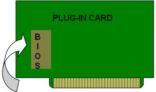
**BIOS** is firmware that's actually part of the device you plug into the system.
