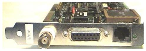
Combination NIC card showing 3 various physical connection types, only RJ-45 is currently used.
