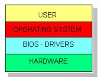
On a computer the **user** interfaces with the **operating system**; the operating system interfaces with hardware through either **BIOS or DRIVERS.**
