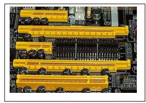
PCIe (top to bottom) PCIe X4 PCIe X16 PCIe X1 PCIe X16 Standard PCI
