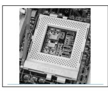
CPU socket and lift the ZIF level to open the socket. Refer to the documentation that came with the CPU to insure that you orient the pins of the CPU so they fit into the socket. Close the ZIF lever to lock the CPU into the socket. Attach the cooling fan to the CPU and follow the manufacturer's suggestion for the heat
