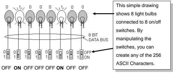
In the above example, **Bit #2** and **Bit #6** are **SET** (turned on), the others are **UNSET** (turned off). We sometimes use the term **SET** to indicate 1 and **UNSET** to indicate 0. The ACSII representation for the upper case "H" is **01000100**, represented by the light bulbs OFF **ON** OFF OFF **ON** OFF OFF.
