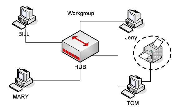
In our small workgroup example, TOM has an attached printer he wants to share on the network. To share an attached printer, open the "**Printers and Faxes**" in the "**Start Menu**", right click on the attached printer, click "**Sharing**" tab.
