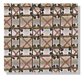
Magnified view shows tiny cores with sensing wires looped through each. Core memory was handmade.
