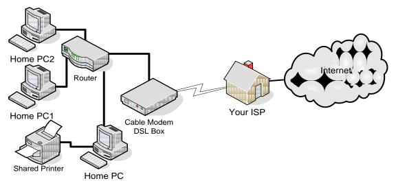
Home user Internet Connection using either Cable Modem, or DSL Box with Router setting up small LAN
