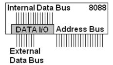
The 8088 has an 8-Bit External Data Bus and a 16-Bit Internal Data Bus.
