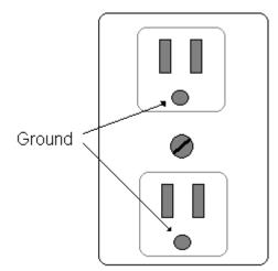
If you use an extension cord to connect your computer to the electrical outlet, make sure the cord has the 3<sup>rd</sup> connector that provides the ground to the system case. The round connector on your power plug is what provides the earth ground that will effectively dissipate any static electricity that might be built up.
