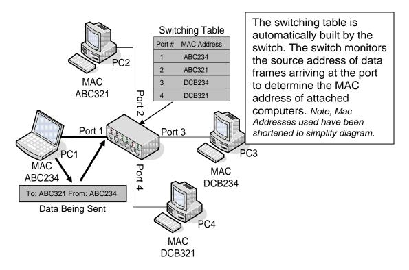
Every NIC card has a unique address that is used for identification on the network; referred to as the MAC address, it is made up of 12 Hexadecimal
