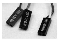
Cables from the front panel are labeled indicating where they plug into the motherboard. Plug the power cable into the ATX connector. If your system does not have integrated video, insert the AGC card and complete the connections from the CD/DVD to the sound card. Make sure cables are dressed properly to allow proper airflow in the system.
