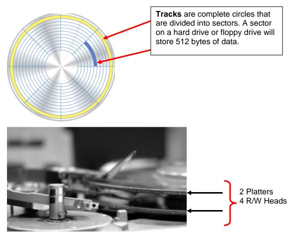
Photo showing the stack of (2) Disk with (4) R/W Heads.
