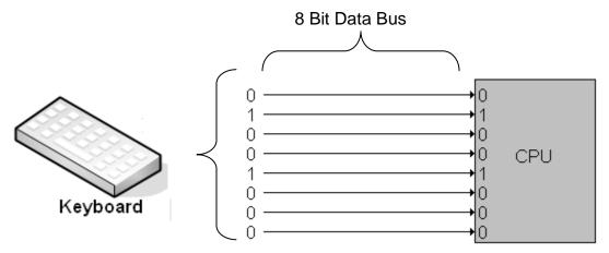
The data bus is conceptually 8 small wires that run from an input device (keyboard) to the CPU. The upper case letter "**H**" represented in ASCII with **01001000** is placed on the bus by the keyboard when the user enters "**Shift h**". To make a Binary **1**, the keyboard places a voltage on the wire; to make a Binary
