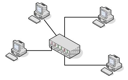
Four PCs connected to a hub using 4 straight through cables
