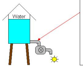
The water in a water tower exerts pressure in the pipe. If the valve is closed, no water will flow and the water wheel will sit motionless.
