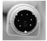
PS/2 connector used for keyboards and mouse connections, also referred to as a 6pin mini-DIN
