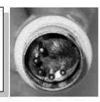
Older systems utilized a 5-pin mini-DIN connector for keyboard.
