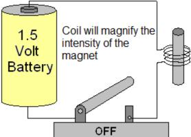
If you wind the wire around a piece of iron, you can create a very powerful Electromagnetic that you can turn on and off by turning on and off the circuit.
