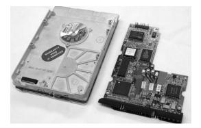
The Controller connects directly to the back of the hard drive.
