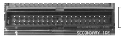
One of the IDE 40 pin connectors on a motherboard.
