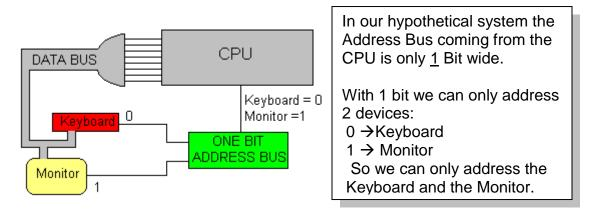
To enable the monitor, the address bus is set to 1; to address the keyboard the bus would be set to 0. So with a one-line address bus we can address two devices, one device with an address of 1 and one device with an address of 0. Now lets see what happens if we double the number of wires used in the Address Bus.
