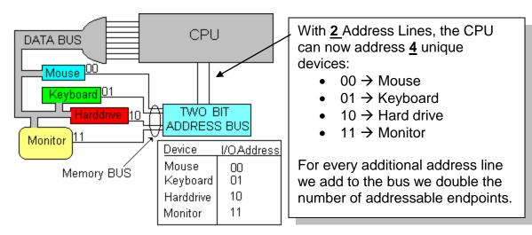
Since we are working with Binary (Base 2), for every line we add to the bus, we double the number of addressable endpoints (the devices we need to access).
