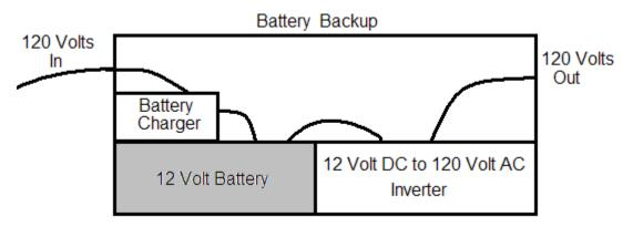
A typical batter back up unit plugs into 120V.A.C., converts that to 12V. D.C. to charge the battery. 12 volts from the battery is fed into an inverter which converts 12V.D.C. back into 120V.A.C.
