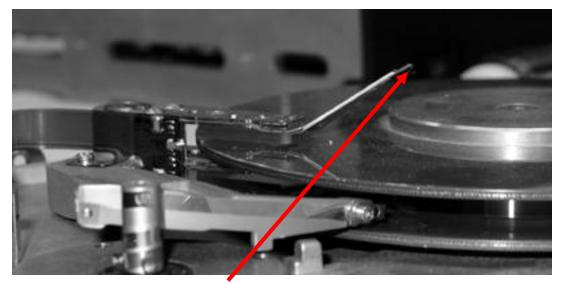
Diagram showing the Read/Write head (bent upward) above one of the hard drive platters. The drive shown above has 2 platters with (4) R/W heads, one for each side.
