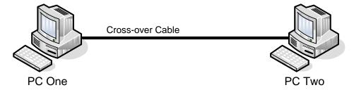
In the above example, **PC One** and **PC Two** are connected together through their NIC cards using a special cross-over cable.
