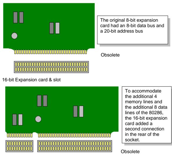
The 8 and 16-bit slot were referred to as an ISA slot, all are now obsolete. New motherboards do not incorporate ISA slots in their design, they had been replaced by a faster expansion bus, PCI which is now being replaced by the PCIe slot.
