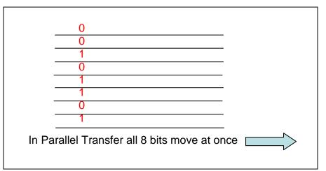
This transfer method worked well at slower speeds, but with new devices running at clock speeds in the GB range the 32 wires that made up the bus, would act like small radio transmitter and introduce noise that would interfere with normal operation. To alleviate the problem parallel transfer is being replaced by serial transfer. With serial transfer, data is sent down a single wire one bit immediately
