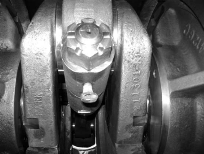
Figure 3-36. Oil Scoop can be seen directly below the bearing cap nut. Courtesy of Power & Compression systems
