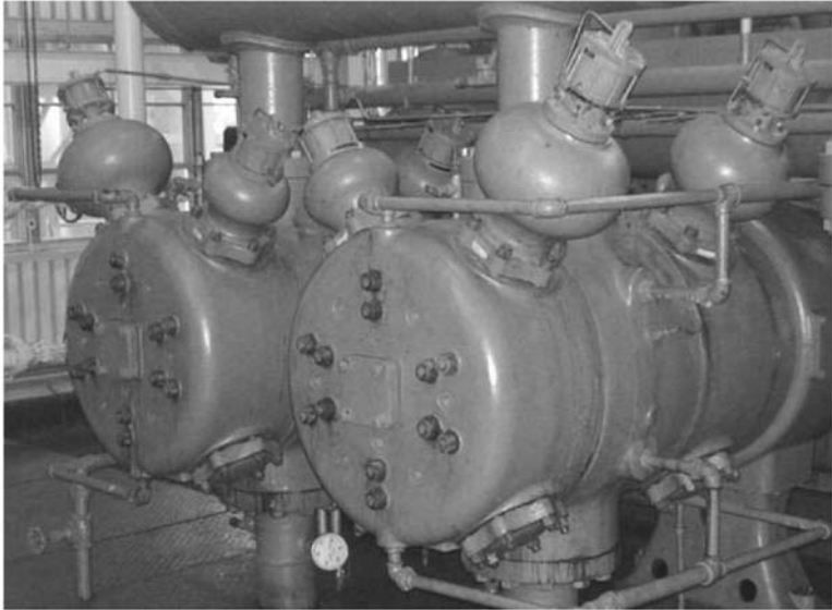
Figure 13-13. Original OEM 1100 psig (75.8 bar) valve-in head type cylinders.
