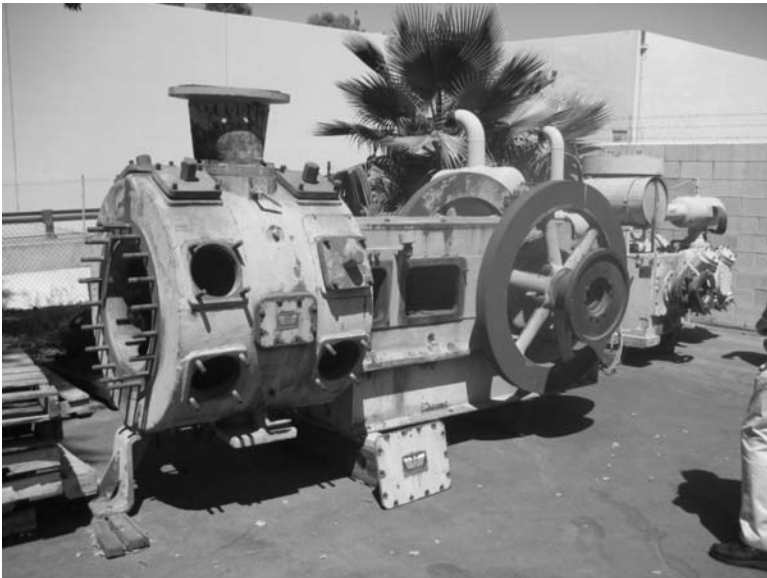
Figure 3-16. Worthington HB GG 24 x 13 Single Stage Compressor before overhaul. Courtesy of Sun Engineering Services, Inc. and Power & Compression Systems Co.
