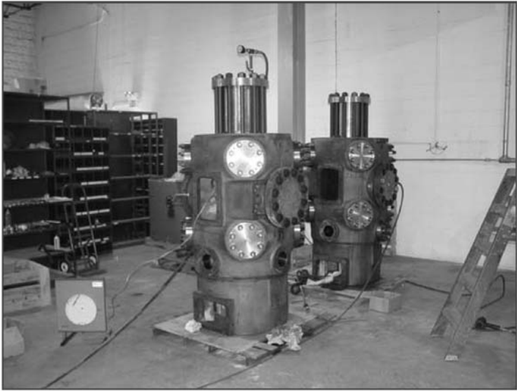
Figure 13-23. Remanufactured cylinders with new fixed volume clearance pocket heads and valve caps undergoing an 8-hr factory hydrostatic test.
