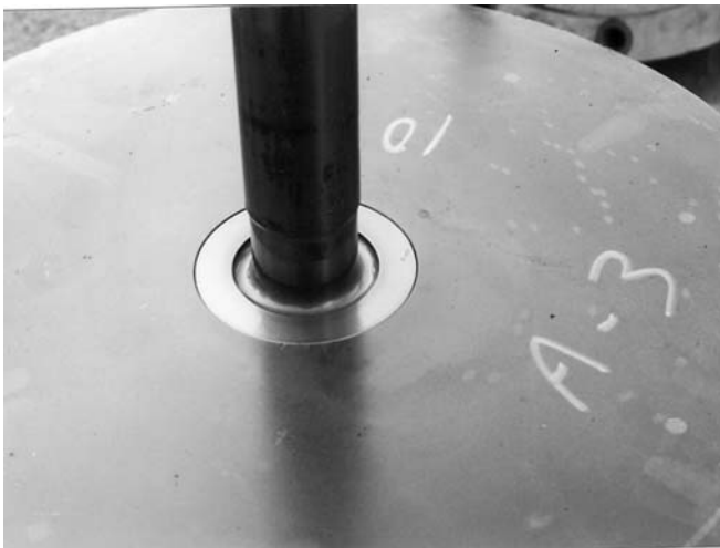
Figure 11-12. Reciprocating Compressor Showing Piston Rod Installed in Crank End of Piston.
