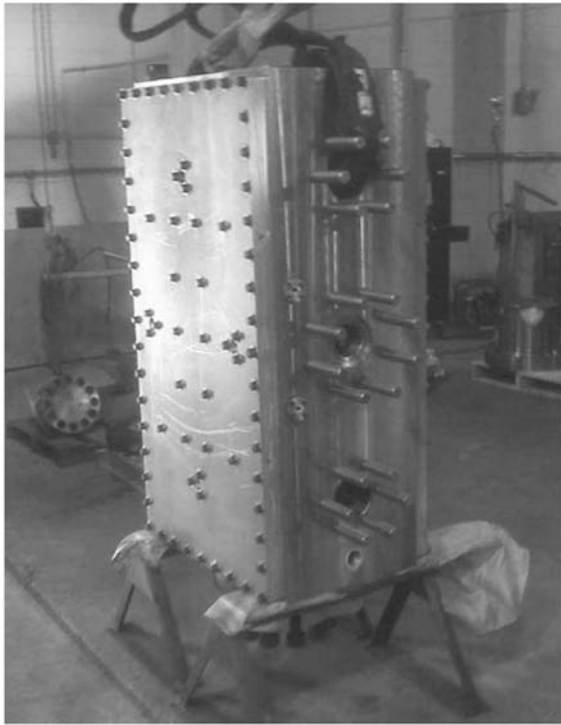
Figure 13-6. New AISI 4140 forged steel cylinder with water jacket, weighing more than 10,000 lb. (4335 kg).
