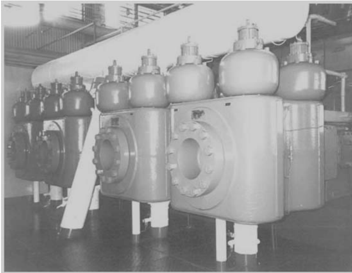
Figure 13-3. Retrofitting custom engineered cylinders increased bore size by 32% on this 17 in. (431.8 mm) stroke Clark integral compressor.
