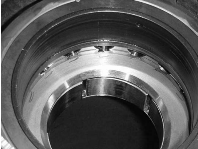
Figure 11-9. Typical Hydrodynamic Tilt-pad Bearing. This Bearing Pivots on Pins Specifically Sized to Obtain the Proper Bearing-to-journal Clearance.
