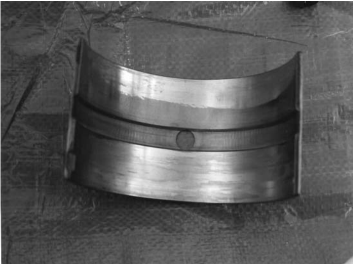
Figure 11-17. Reciprocating Compressor Hydrodynamic Bearing Shoe Showing Normal Wear.
