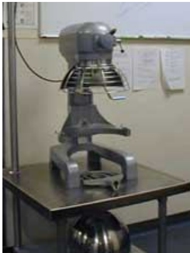
Fig 4.3 Mixer with machine guarding
