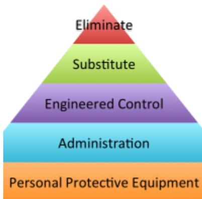
The hierarchy of control is a risk management process. It is a system used in industry to minimize or eliminate exposure to hazards.
