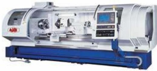
**CNC lathe:** Substituting a centre lathe with a CNC lathe (Computer Numeric Control) is an example of improved risk control of machinery and equipment through improvement in design.
