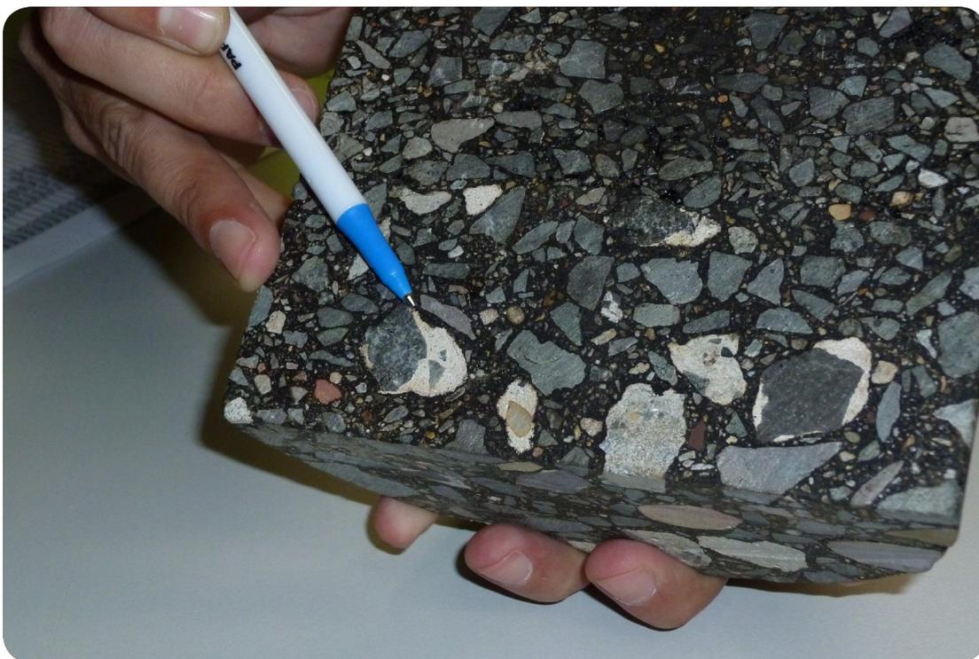
65% Recycled asphalt showing recycled material aggregate.
