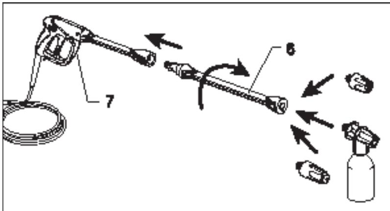
1. Push the spray lance (6) into the spray gun (7) and twist it until the bayonet coupling locks into position.
