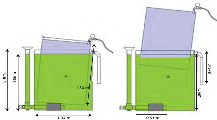
ARTI design compact biogas plant, made from one 750-litre and one 1000-litre water tank (Riuzzi, 2009)
