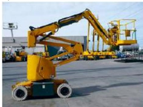
**Note:** Safe work practices must take into account the risk of trapping an operator between the EWP and a fixed structure (e.g. overhead beams, electrical cables, pipes).
