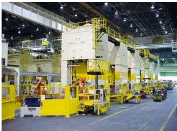
Permanently fixed gantries, ladders and walkways are incorporated into this machinery and equipment to reduce the risk of a fall from height occurring during operation and maintenance.
