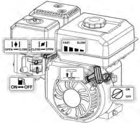
1. Turn the engine switch to "ON" position.
