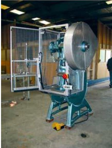
An old style press refurbished with an interlocked safety cage and gate.
