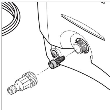
Clean the water inlet filter regularly once a month or more frequently according to use. Carefully loosen the filter with a screwdriver and clean it. Check that it is intact before re-mounting it.
