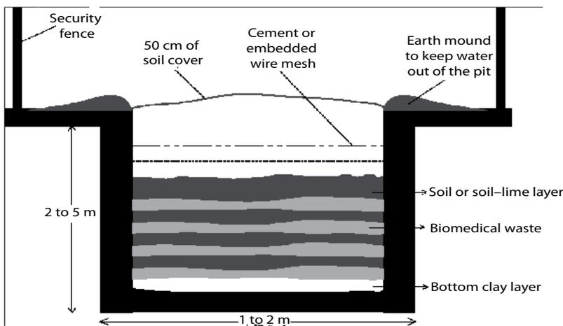
Figure 14.1 Construction of a pit for onsite waste burial
