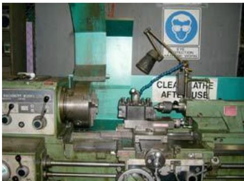
**Centre lathe:** The exposed rotating chuck of a centre lathe can eject parts or tools with great force, cutting fluid fumes are difficult to contain and the machinery requires manual set-up.
