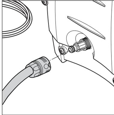
**IMPORTANT! Only use water without any impurities.** If there is a risk of silt, sand or sediment in the inlet water (i.e. from your own well), an additional filter (106411231) should be mounted.
