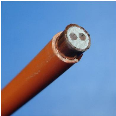
Figure F-6-1-1(c) Mineral Insulated Metal Sheathed cable (MIMS)
