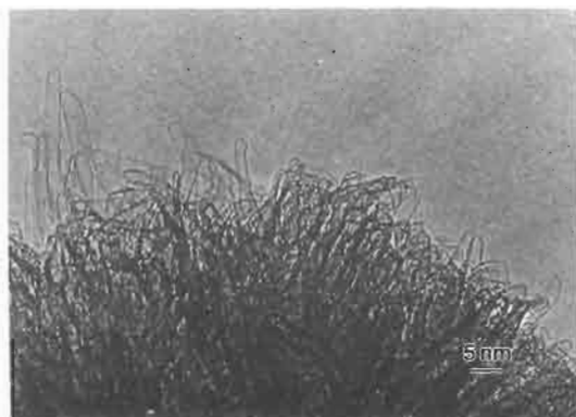
Fig. 4. Various morphologies of single-shell buckytubes.
