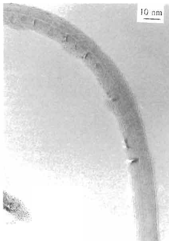
Figure 3. Lattice fringes LF 002 of buckled nanotube particles.
