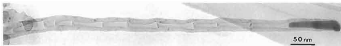
Fig. 8. TEM picture of a bamboo-shaped carbon tube.
