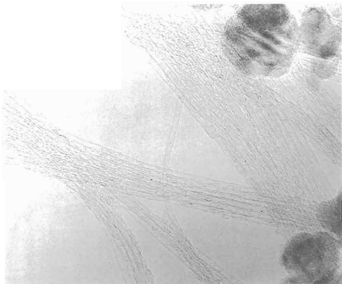
Fig. 2. Cables of parallel SWNTs that have self-assembled during oxidative cleanup of arc-produced soot composed of randomly oriented SWNTs imbedded in amorphous carbon. Note the large cable consisting of several tens of SWNTs, triple and single strand tubes bent without kinks, and another bent cable consisting of 6 to 8 SWNTs.
